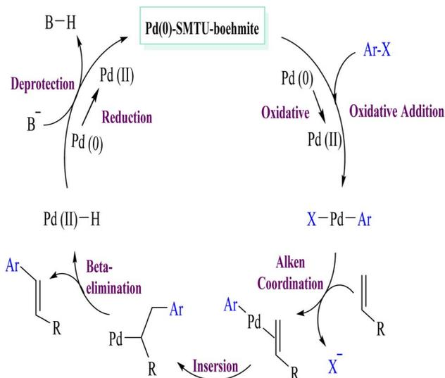
**Scheme 5** Proposed mechanism of the Mizoroki–Heck reaction involving Pd(0)-SMTU-boehmite.
