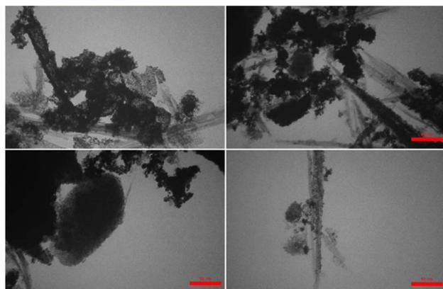
**Fig. 6** TEM image of Pd(0)-SMTU-boehmite nanoparticles.
