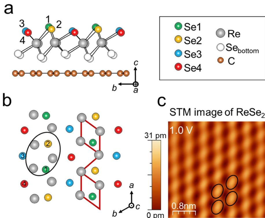
**Fig. 1** Monolayer (ML)  $\text{ReSe}_2$  on a graphene substrate. (a and b) The side- and top-view structures of ML  $\text{ReSe}_2$ . The Se atoms in the topmost layer are classified into Se1 (green), Se2 (orange), Se3 (blue), and Se4 (red) based on their height along the  $c$ -axis. The Re-chain is indicated by red solid lines in (b). (c) The STM topography image of  $\text{ReSe}_2$  shows the oval feature with a lattice constant of  $\sim 6.6 \text{ \AA}$  ( $I_t = 30 \text{ pA}$ ).
