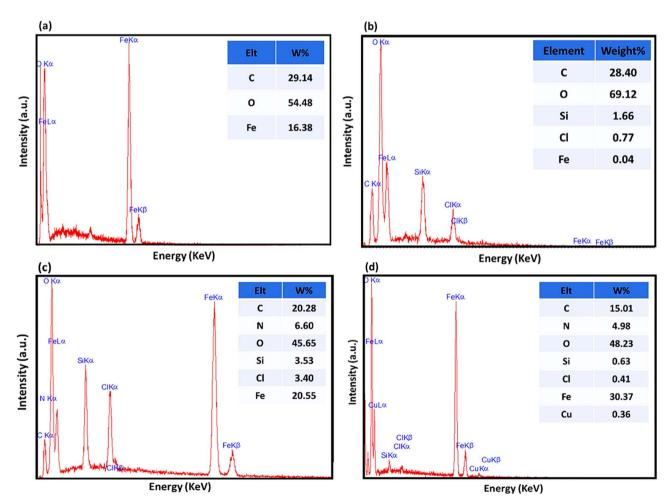
Fig. 2 Results of the energy dispersive X-ray (EDX) analysis of Fe<sub>3</sub>O<sub>4</sub>@AG (a), Fe<sub>3</sub>O<sub>4</sub>@AG@CPTMS (b), Fe<sub>3</sub>O<sub>4</sub>@AG/AP (c), and Fe<sub>3</sub>O<sub>4</sub>@AG/AP-Cu(ı) (d) nanocomposites.
