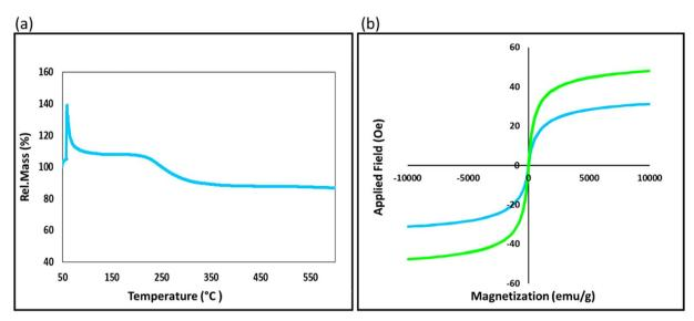
Fig. 3 The TGA of the Fe<sub>3</sub>O<sub>4</sub>@AG/AP-Cu(i) nanocomposite (a), and the M-H curves of the Fe<sub>3</sub>O<sub>4</sub>@AG (green curve) and Fe<sub>3</sub>O<sub>4</sub>@AG/AP-Cu(i) nanocomposites (blue curve) at room temperature (b).
