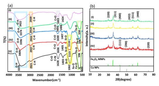
$\label{eq:Fig.1} FIIR spectra of AG (I), Fe_3O_4@AG (II), Fe_3O_4@AG(CPTMS (III), Fe_3O_4@AG/AP (IV), and Fe_3O_4@AG/AP-Cu(i) (V) (a) and XRD patterns of Fe_3O_4@AG (I), Fe_3O_4@AG(CPTMS (III), Fe_3O_4@AG/AP-Cu(i) (IV) nanocomposites (b).$
