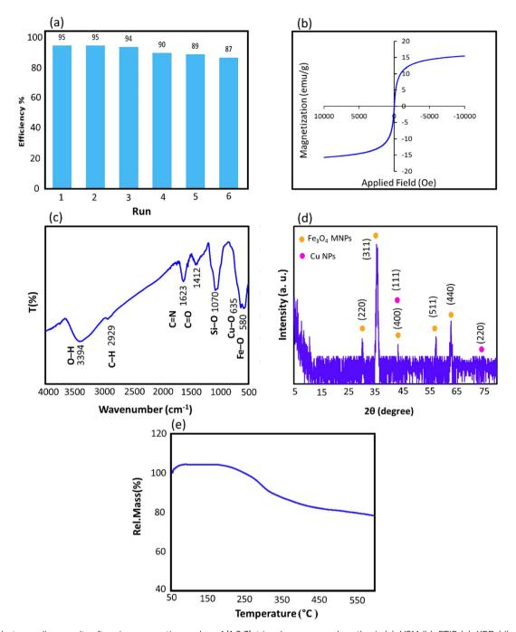
Fig. 5 Catalyst recycling results after six consecutive cycles of [1,2,3]-triazole compound synthesis (a), VSM (b), FTIR (c), XRD (d), and TGA (e) analyses of the nanocatalyst after six sequential recycling cycles.
