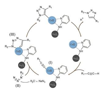
Scheme 2 The synthesis reaction mechanism of triazole derivatives in the presence of the  $Fe_3O_4@AG/AP-Cu(i)$  nanocomposite.
