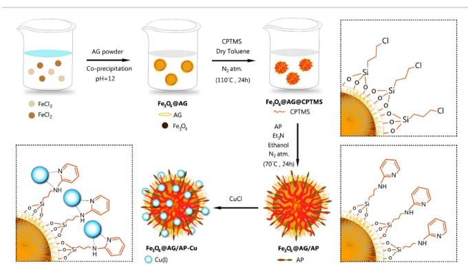
Scheme 1 The preparation process of the Fe<sub>3</sub>O<sub>4</sub>@AG/AP-Cu(ı) magnetic nanocomposite.
