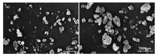
FESEM images of the nanocatalyst after six sequential recycling cycles on two scales, 1.0 μm (a) and 700.0 nm (b).
