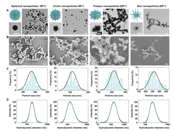
Fig. 1 Characterization of four structural DNA nanoparticles. (A) TEM images and (B) SEM images of the four structural DNA nanoparticles. Scale bar: 200 nm. (C) Diameter distribution of DNA nanostructures measured from TEM images. (D) Hydrodynamic diameter distribution of DNA nanostructures in an aqueous solution measured by DLS.
