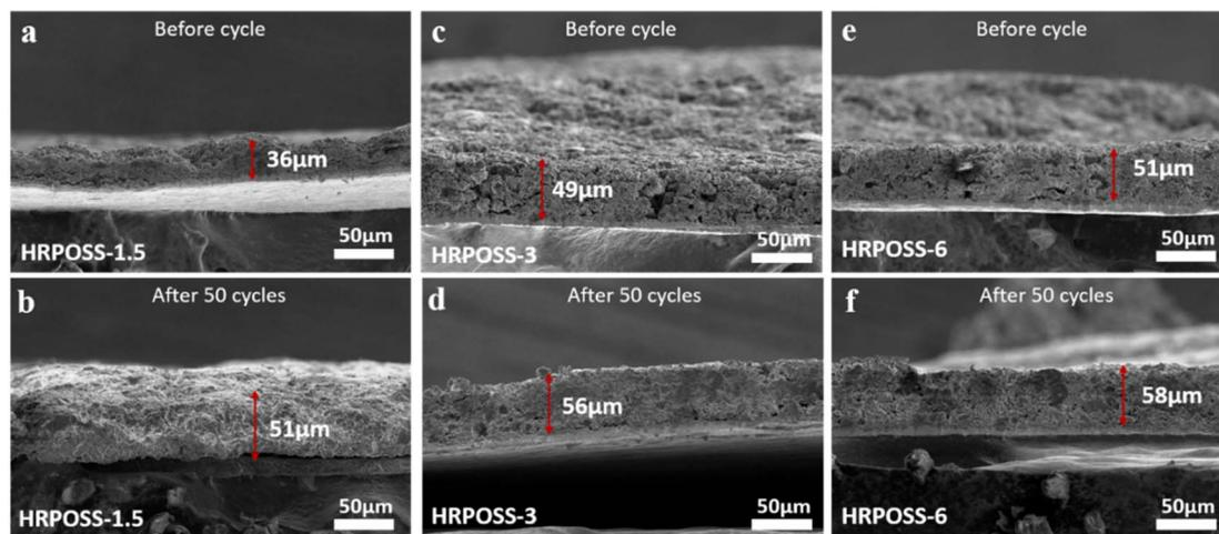
Fig. 6 Series of SEM images showing the electrode changes before and after 50 cycles. Cross-sectional view of HRPOSS-1.5, HRPOSS-3 and HRPOSS-6 electrodes before cycling (a, c, and e) and after 50 cycles (b, d, and f), respectively (cross section of the electrode was taken from two halves of the same electrode).
