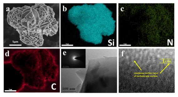
Fig. 3 SEM images of (a) HRPOSS-6 and corresponding EDS elemental mapping images of (b) Si, (c) N, and (d) C, (e) TEM image and corresponding SAED pattern of HRPOSS-6, and (f) HRTEM image of HRPOSS-6.
