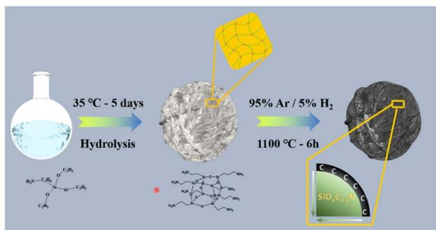
Fig. 1 Schematic diagram for the synthesis of HRPOSS.
