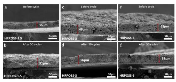
Fig. 6 Series of SEM images showing the electrode changes before and after 50 cycles. Cross-sectional view of HRPOSS-1.5, HRPOSS-3 and HRPOSS-6 electrodes before cycling (a, c, and e) and after 50 cycles (b, d, and f), respectively (cross section of the electrode was taken from two halves of the same electrode)
