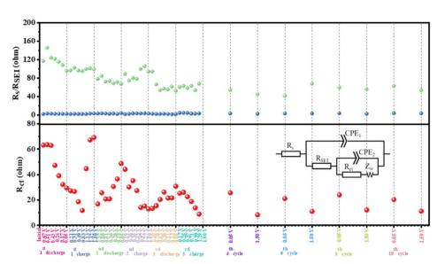
Fig. 8 Fitted results of electrolyte resistance,  $R_{sr}$  resistance of the SEI layer,  $R_{SFI}$ , and charge-transfer resistance,  $R_{ct}$ . Inset: corresponding equivalent electrical circuit
