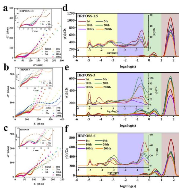
Fig. 7 EIS characterization of the electrodes. Nyquist plots of after various cycles in (a) HRPOSS-1.5, (b) HRPOSS-3 and (c) HRPOSS-6 electrode. Distribution of relaxation time-related function  $\gamma(\tau)$  after various cycles of (d) HRPOSS-1.5, (e) HRPOSS-3 and (f) HRPOSS-6 electrode.
