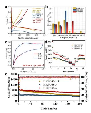
Fig. 5 (a) Initial charge/discharge voltage profiles. (b) Capacity distribution in different voltage ranges. (c) CV curves. (d) Rate performance. (e) Long-term cycle performance at 500 mA  $\rm g^{-1}$  of HRPOSS-1.5, HRPOSS-3 and HRPOSS-6
