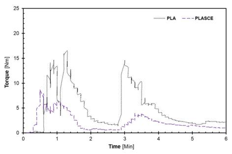
Fig. 1 A plot of torque vs. time plots during melt-mixing of PLA and plasticized PLA; (a) first, and (b) second mixing regimen.
