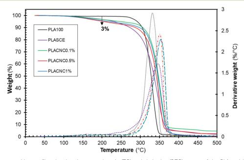
Fig. 9 Thermal decomposition profiles showing thermogravimetric (TG) and derivative (DTG) curves of the PLA and bionanocomposites filaments.
