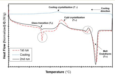
Fig. 10 DSC thermograms of the neat PLA filaments showing the first, cooling and second heating runs.
