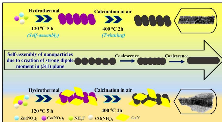
Scheme 1 Formation mechanism displaying the synthesis scheme.
