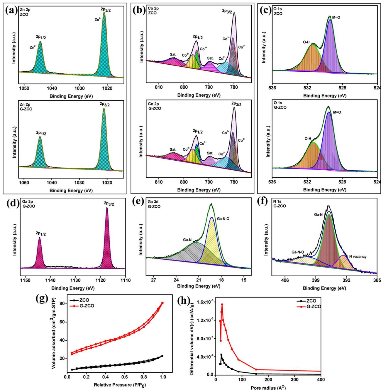
Fig. 2 High-resolution deconvoluted XPS analysis of (a) Zn, (b) Co, and (c) O of ZCO and G-ZCO, and (d) Ga 2p, (e) Ga 3d, and (f) N 1s of G-ZCO. (g) Isotherm plots and the (h) corresponding pore size distribution for ZCO and G-ZCO.
