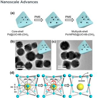
Fig. 9 (a) Schematic illustration for the localized oxidative linker cleaving process; (b and c) TEM images of (b) core–shell Pd@UiO-66-(OH)<sub>2</sub> and (c) multiyolk–shell NPNS@MOF nanostructures; (d) schematic illustration of the oxidative linker cleaving process catalyzed by Pd nanoparticles in core–shell Pd@UiO-66-(OH)<sub>2</sub> nanoparticles (abbreviations: PMS = peroxymonosulfate; DOBDC = 2,5-dihydroxyterephthalic acid) (Copyright 2019, American Chemical Society).<sup>60</sup>
