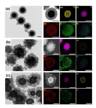
Fig. 16 TEM image and the corresponding EDX elemental mapping data for (a) rattle-type Au-NPNS@Zn-MOF nanohybrids, and (b and c) rattle-type Au-NPNS@ZIF-8 nanohybrids with different particle sizes of Au nanoparticles, showing gold (in yellow), silica (in purple), zinc (in red), carbon (in green), and nitrogen (in blue). Scale bar: 500 nm, (Copyright 2020, Springer Nature).<sup>73</sup>
