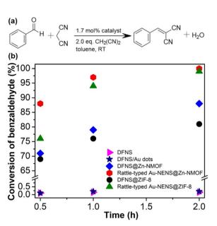
Fig. 22 (a) Knoevenagel condensation reaction scheme and (b) the conversion of benzaldehyde *versus* reaction time, using DFNS (in pink), DFNS/Au dots (in navy), DFNS@Zn-NMOF (blue), rattle-type Au-NPNS@Zn-NMOF (red), DFNS@ZIF-8 (in black), and rattle-type Au-NPNS@ZIF-8 (in dark green) as catalysts. The catalyst quantity is 1.7 mol% (Copyright 2020, Springer Nature).<sup>73</sup>
