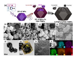
Fig. 24 (a) Schematic illustration of the formation process of CoP@-FeCoP/NC YSMPs. (b-d) SEM images of (b) ZIF-67 MPs, (c) CoP/NC NPs, and (d) ZIF-67@Co-Fe PBA YSMPs. Insets of (b-d) show the corresponding TEM images. (e) SEM, (f and g) TEM and (h) HR-TEM images of CoP@FeCoP/NC YSMPs. (i) HAADF-STEM and elemental mapping images for Co, Fe, P, N, and C of CoP@FeCoP/NC YSMPs (Copyright 2021, Elsevier).98
