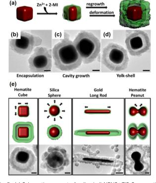
Fig. 3 (a) Schematic concept of yolk-shell NPNS@ZIF-8 generation with a cubic hematite crystal as the core and ZIF-8 as the shell, (b-d) TEM images of the growth pathway, and (e) schematic illustrations of the dominant deformation directions during shell growth (top) and yolk-shell architecture generation (middle), accompanied by TEM images (bottom). Scale bars: 500 nm (Copyright 2014, American Chemical Society).48
