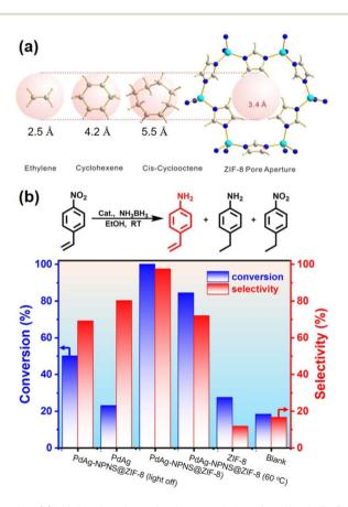
Fig. 20 (a) Molecular-size-selective catalysis of yolk-shell Pd-NPNS@MOF<sup>47</sup> and (b) chemoselective hydrogenation of *para*-nitro-styrene over PdAg-NPNS@ZIF-8 and different catalysts<sup>46</sup> (Copyright 2012 and copyright 2022, American Chemical Society).
