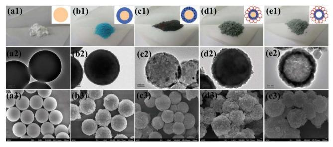
Fig. 18 The photographic (top row), TEM (middle row), and SEM (bottom row) images for (a) SPS, (b) SPS@HKUST-1, (c) SPS@HKUST-1/Pd, (d) SPS@HKUST-1/Pd@ZIF-8, and (e) Pd-NPNS@HKUST-1@ZIF-8 nanohybrids. The scale bars are 200 nm for TEM and 100 nm for SEM images, respectively (Copyright 2017, Wiley-VCH).80
