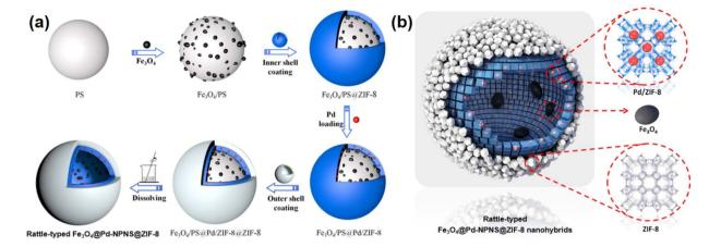
Fig. 13 (a) Schematic illustration for the fabrication and (b) structural compositions of rattle-type  $Fe_3O_4$ @Pd-NPNS@ZIF-8 nanoarchitectures (Copyright 2019, American Chemical Society).<sup>72</sup>
