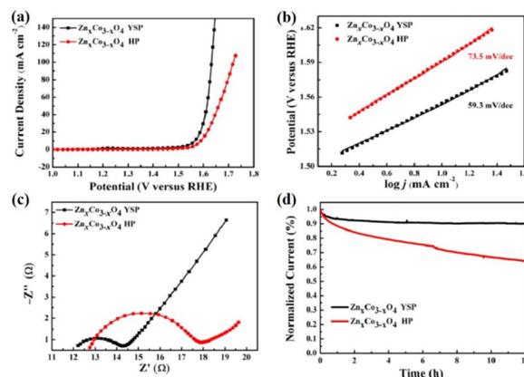
Fig. 26 (a) Linear sweep voltammety curves and (b) Tafel plots of  $Zn_xCo_{3-x}O_4$  YSP and  $Zn_xCo_{3-x}O_4$  HP in an  $O_2$ -saturated 1 M KOH electrolyte. (c) Nyquist plots of  $Zn_xCo_{3-x}O_4$  YSP and  $Zn_xCo_{3-x}O_4$  HP. (d) Time-dependent current densities of  $Zn_xCo_{3-x}O_4$  YSP and  $Zn_xCo_{3-x}O_4$  HP (Copyright 2017, American Chemical Society).<sup>99</sup>
