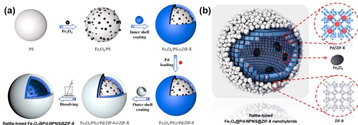
Fig. 13 (a) Schematic illustration for the fabrication and (b) structural compositions of rattle-type Fe<sub>3</sub>O<sub>4</sub>@Pd-NPNS@ZIF-8 nanoarchitectures (Copyright 2019, American Chemical Society).<sup>72</sup>
