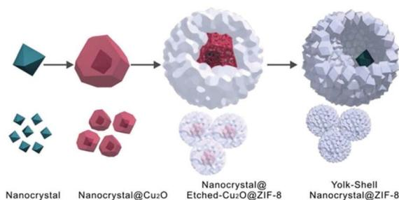
Fig. 2 Schematic growth procedure for the yolk-shell NPNS@ZIF-8 nanostructure (Copyright 2012, American Chemical Society).<sup>47</sup>
