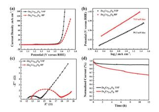
Fig. 26 (a) Linear sweep voltammetry curves and (b) Tafel plots of  $Zn_xCo_{3-x}O_4$  YSP and  $Zn_xCo_{3-x}O_4$  HP in an  $O_2$ -saturated 1 M KOH electrolyte. (c) Nyquist plots of  $Zn_xCo_{3-x}O_x$  YSP and  $Zn_xCo_{3-x}O_4$  HP. (d) Time-dependent current densities of  $Zn_xCo_{3-x}O_4$  YSP and  $Zn_x-Co_{3-x}O_4$  HP (Copyright 2017, American Chemical Society).<sup>99</sup>
