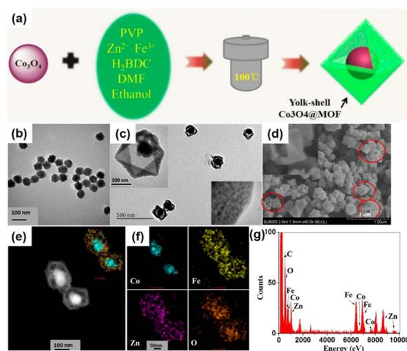
Fig. 6 (a) Synthetic strategy for yolk-shell  $\text{Co}_3\text{O}_4$ -NPNS@MOF nanostructures; TEM images of (b)  $\text{Co}_3\text{O}_4$  nanoparticles and (c) yolk-shell  $\text{Co}_3\text{O}_4$ -NPNS@MOF nanostructures; (d) SEM image, (e) HAADF-STEM image, (f) elemental mapping, and (g) EDX spectra of yolk-shell  $\text{Co}_3\text{O}_4$ -NPNS@MOF nanostructures. The insets in (c) show the closer TEM observation (Copyright 2015, American Chemical Society).<sup>56</sup>
