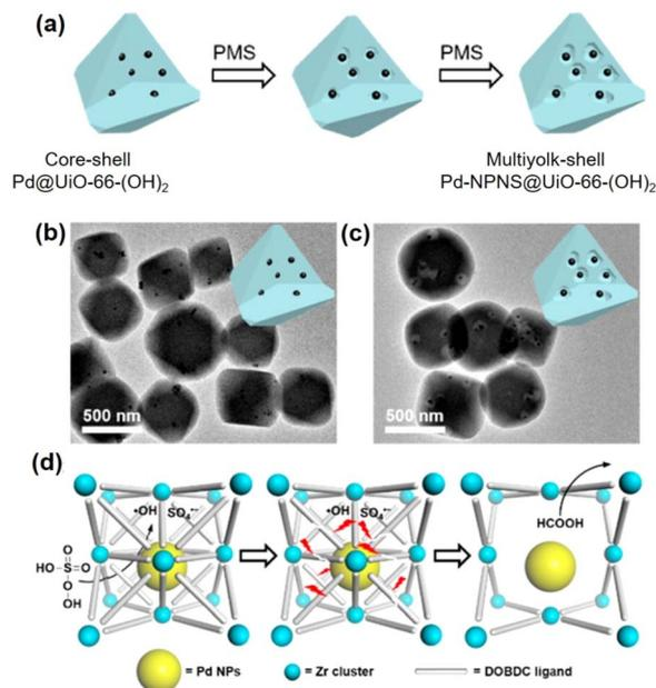
Fig. 9 (a) Schematic illustration for the localized oxidative linker cleaving process; (b and c) TEM images of (b) core-shell Pd@UiO-66-(OH)<sub>2</sub> and (c) multiyolk-shell NPNS@MOF nanostructures; (d) schematic illustration of the oxidative linker cleaving process catalyzed by Pd nanoparticles in core-shell Pd@UiO-66-(OH)<sub>2</sub> nanoparticles (abbreviations: PMS = peroxymonosulfate; DOBDC = 2,5-dihydroxyterephthalic acid) (Copyright 2019, American Chemical Society).<sup>60</sup>
