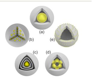
Fig. 1 Schematic illustration of different NPNS@MOF hybrid nanomaterials: (a) yolk-shell, (b) multiyolk-shell, (c) yolk-multishell, (d) rattle-type, and (e) dot-in-shell NPNS@MOF nanoarchitectures.
