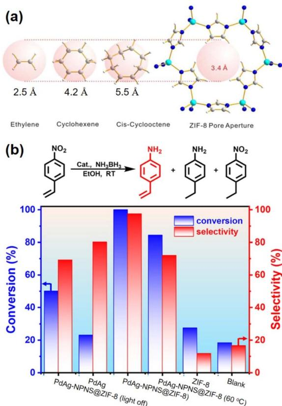
Fig. 20 (a) Molecular-size-selective catalysis of yolk-shell Pd-NPNS@MOF<sup>47</sup> and (b) chemoselective hydrogenation of *para*-nitrostyrene over PdAg-NPNS@ZIF-8 and different catalysts<sup>46</sup> (Copyright 2012 and copyright 2022, American Chemical Society).
