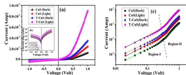
Fig. 10 (a) Current–voltage (*I*-*V*) plots, (b) log scale *I* vs. *V* curves and (c) log *I*-log *V* plot of the bare CuS and T-CuS composite-based Schottky diodes under dark and illumination conditions.
