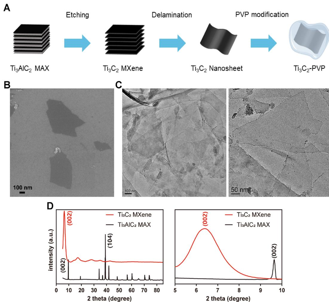
Fig. 1 Characterization. (A) Schematic of the preparation of  $\text{Ti}_3\text{C}_2$  MXene nanosheets and PVP modification. (B) SEM image of  $\text{Ti}_3\text{C}_2$  nanosheets. (C) TEM images of  $\text{Ti}_3\text{C}_2$  nanosheets. (D) XRD pattern of  $\text{Ti}_3\text{AlC}_2$  MAX and  $\text{Ti}_3\text{C}_2$  MXene.
