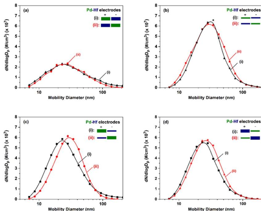
**Fig. 3** Particle size distributions, measured by the SMPS, of the Pd–Hf NPs produced by the SDG when using pairs of (a) thick electrodes, (b) thin electrodes, (c) a thin Hf and a thick Pd electrode, and (d) a thin Pd and a thick Hf electrode. For each case, comparison of the size distributions is made when switching the polarity of the electrode pairs. The thick and thin electrodes used in our measurements had diameters of 2 and 0.25 mm, respectively.
