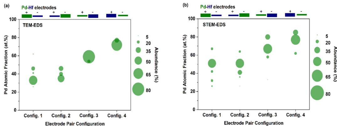
Fig. 7 Fraction of Pd (at%) in the mixed, (a) agglomerated (determined by TEM-EDS), and (b) primary (determined by STEM-EDS) particles produced by the SDG when using different electrode pair configurations. In all cases, the thick and thin electrodes had diameters of 2 and 0.25 mm, respectively.
