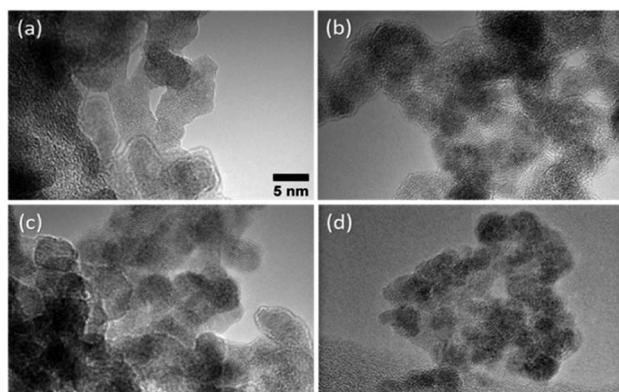
**Fig. 4** TEM images of Pd–Hf agglomerates produced by the SDG when using the following electrode configurations: (a) a thick-positive Pd and a thin-negative Hf electrode, (b) a thick-negative Pd and a thin-positive Hf electrode, (c) a thin-positive Pd and a thick-negative Hf electrode, and (d) a thin-negative Pd and a thick-positive Hf electrode. In all cases, the thick and thin electrodes had diameters of 2 and 0.25 mm, respectively.
