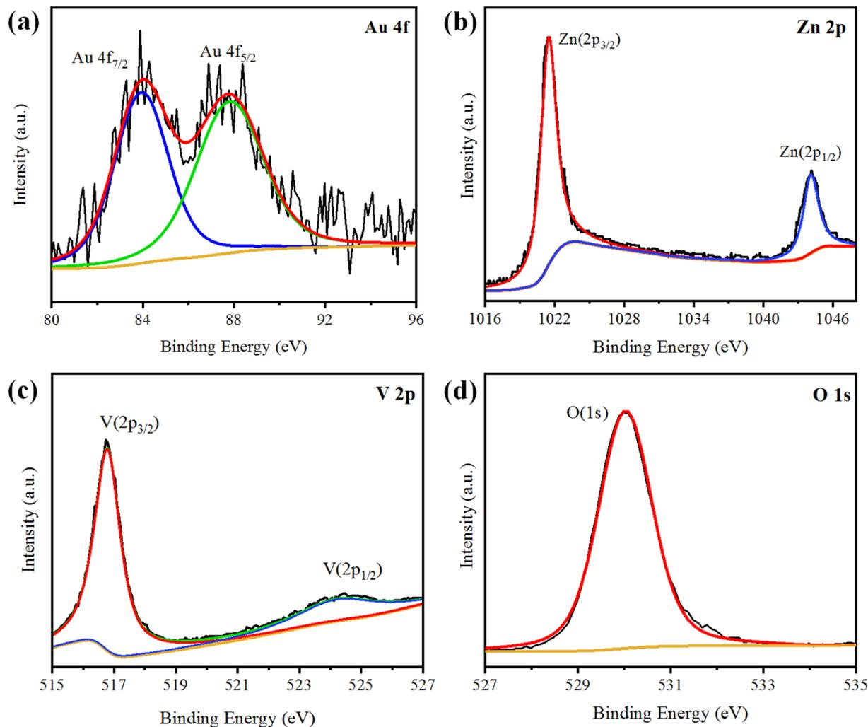
Fig. 4 XPS results of Au@Zn<sub>3</sub>V<sub>2</sub>O<sub>8</sub> showing: (a) Au 4f, (b) Zn 2p, (c) V 2p, and (d) O 1s plots.
