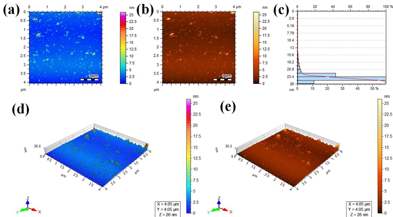
Fig. 5 AFM results: (a and b) 2D tapping modes, (c) size distribution, and (d and e) 3D images of the Au@Zn<sub>3</sub>V<sub>2</sub>O<sub>8</sub> photocatalysts.
