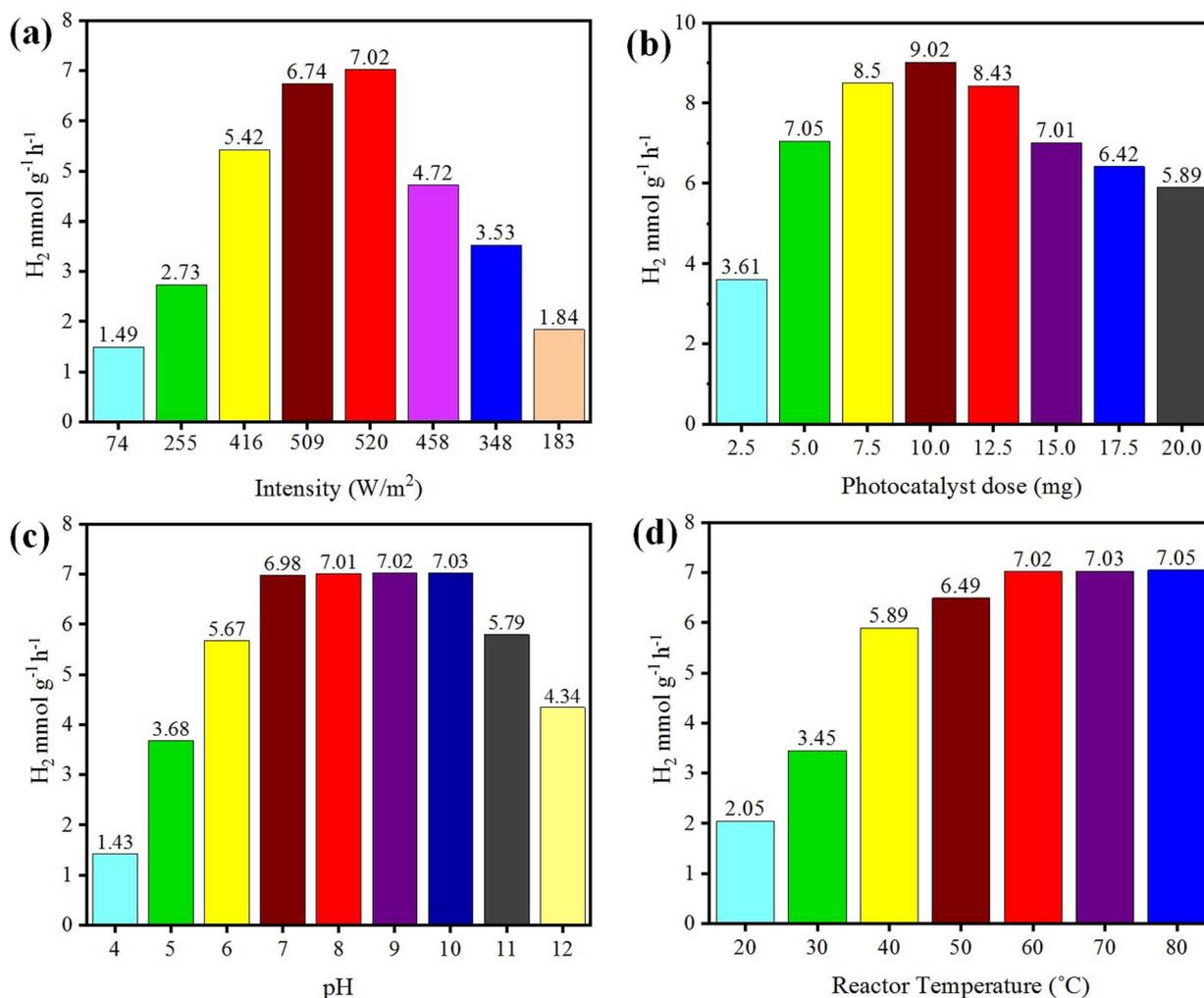
Fig. 9 Effects of (a) intensity, (b) concentration, (c) pH, and (d) temperature on photocatalytic H<sub>2</sub> generation.
