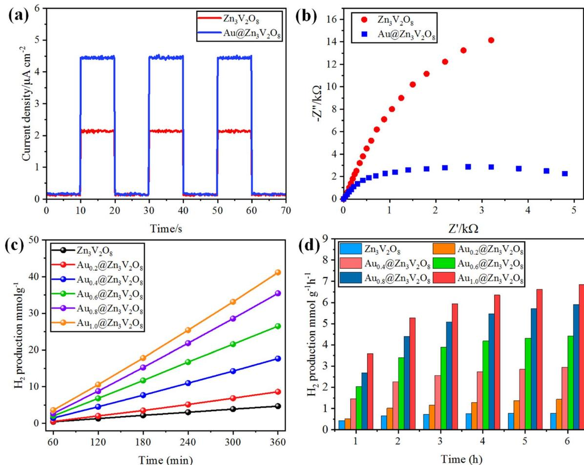
Fig. 7 (a) Photocurrent response, (b) EIS results of  $\text{Zn}_3\text{V}_2\text{O}_8$  and  $\text{Au@Zn}_3\text{V}_2\text{O}_8$ . (c and d) comparison of the photocatalytic activities of the photocatalysts in  $\text{mmol g}^{-1}$  and  $\text{mmol g}^{-1} \text{h}^{-1}$ , respectively.
