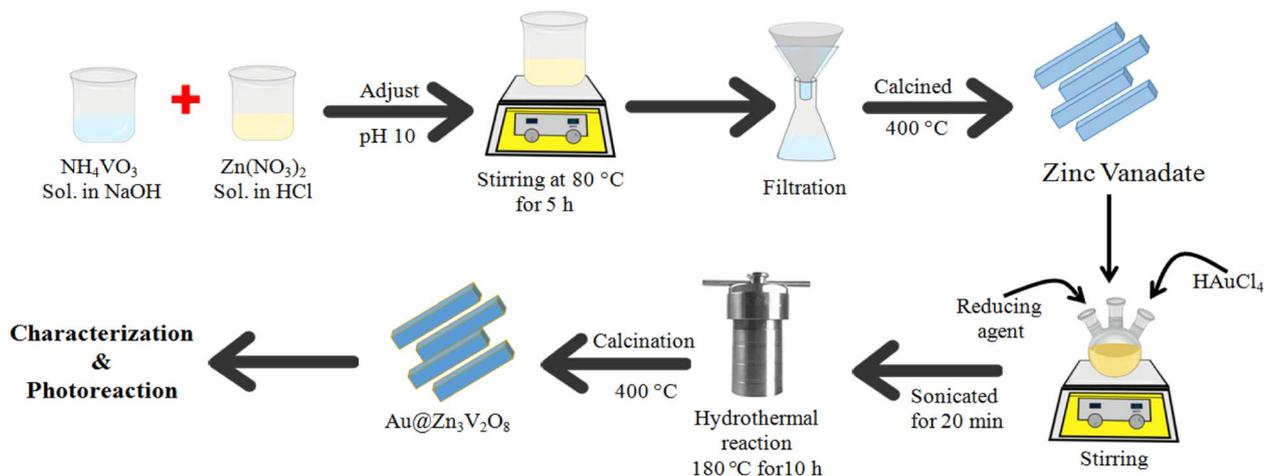
Fig. 1 Illustration of the synthesis of the  $\text{Zn}_3\text{V}_2\text{O}_8$  and  $\text{Au}@Z\text{n}_3\text{V}_2\text{O}_8$  catalysts.
