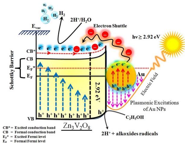
Fig. 8 Illustration of SPR electron transfer for photocatalytic H<sub>2</sub> evolution.
