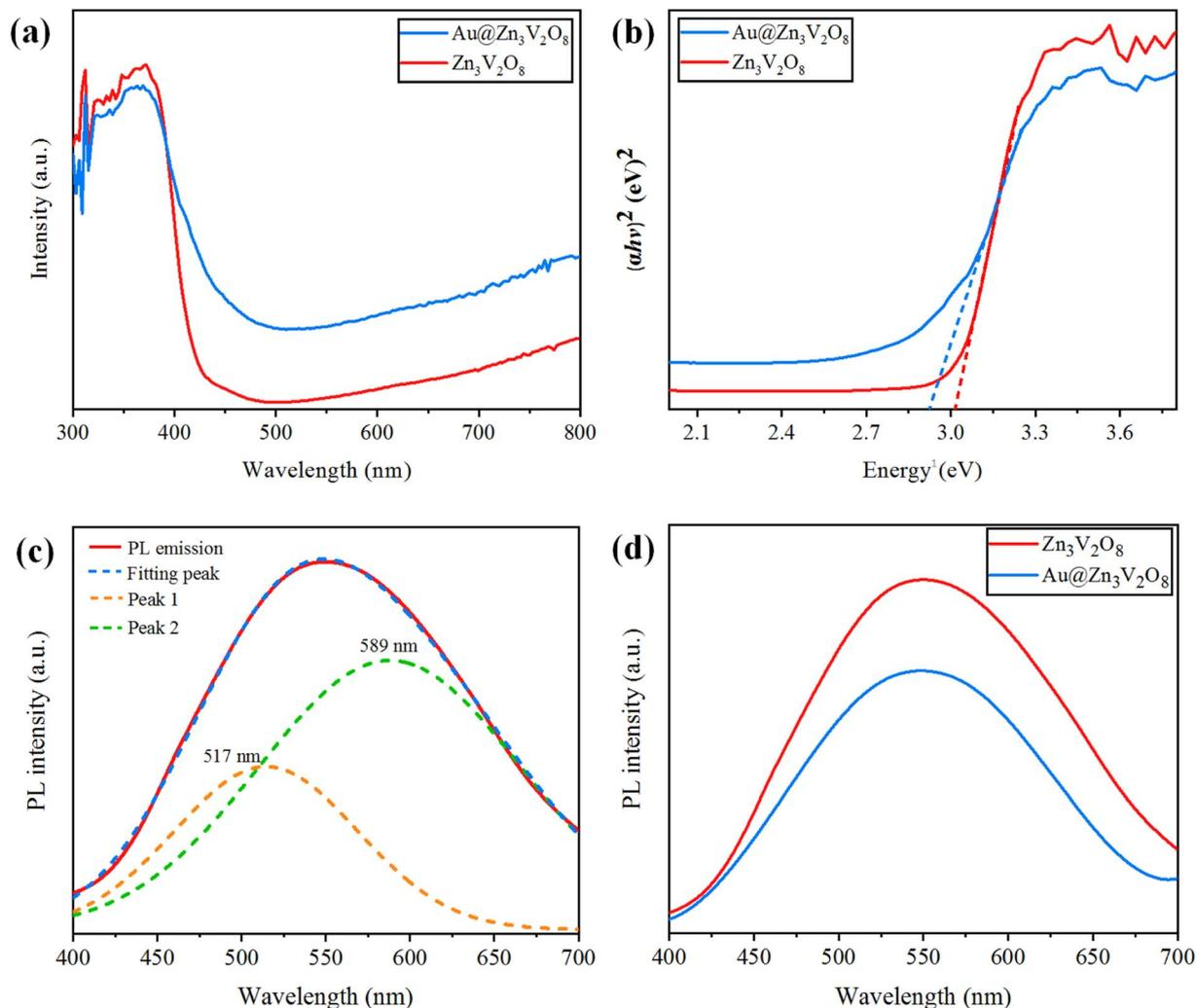
Fig. 6 (a) UV-Vis-DRS, (b) energy curves (eV), (c) PL emission spectra and fitting of the peaks, and (d) PL emission spectra for the  $\text{Z}_3\text{V}_2\text{O}_8$  and  $\text{Au}@Z_3\text{V}_2\text{O}_8$  catalysts.
