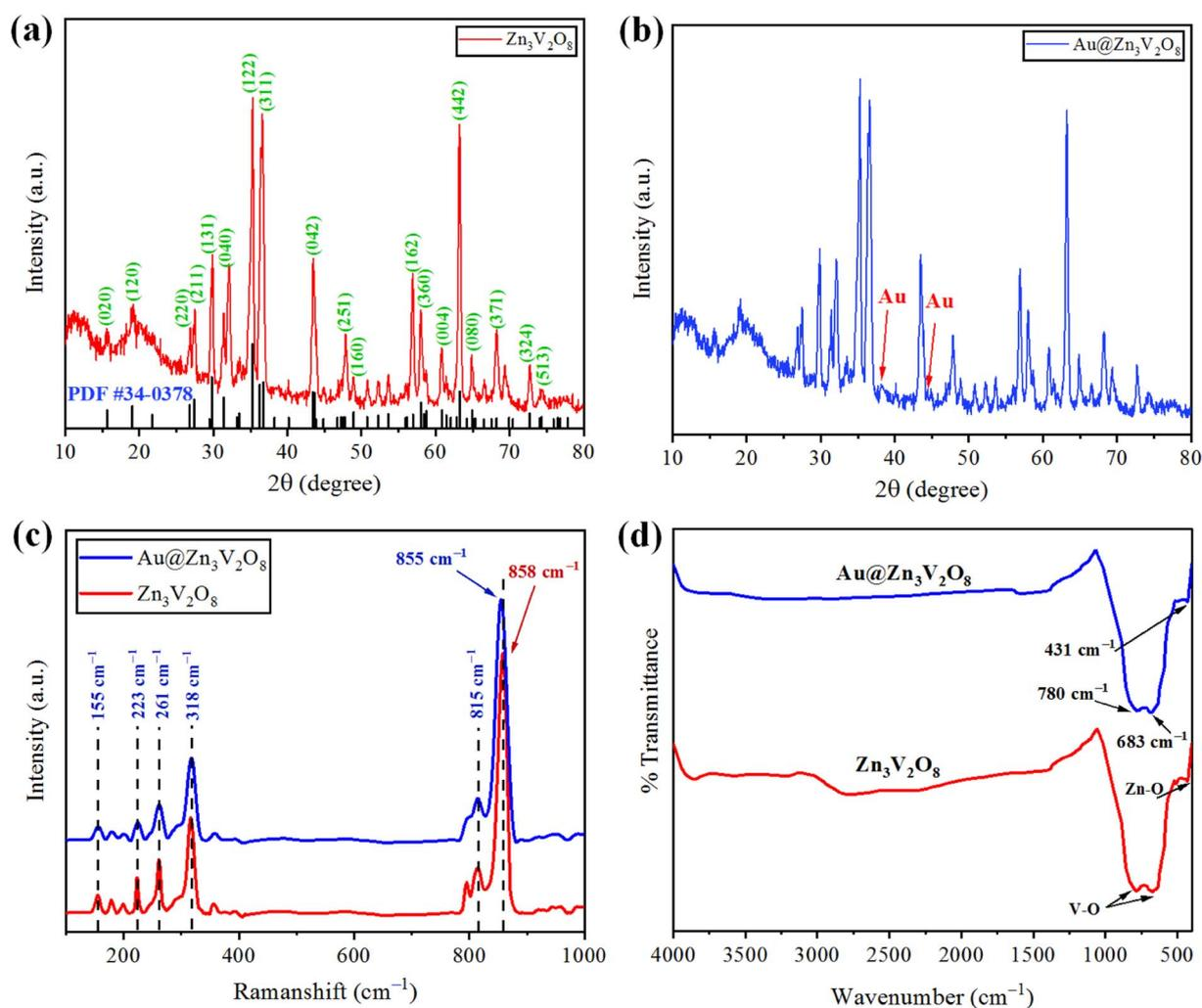
Fig. 2 (a and b) XRD patterns of  $\text{Zn}_3\text{V}_2\text{O}_8$  and  $\text{Au}@Z\text{n}_3\text{V}_2\text{O}_8$  catalysts. (c and d) Raman and FTIR results of pure  $\text{Zn}_3\text{V}_2\text{O}_8$  and  $\text{Au}@Z\text{n}_3\text{V}_2\text{O}_8$ , respectively.
