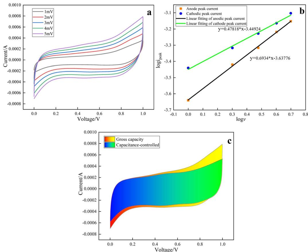
Fig. 11 Analysis diagram of the  $\epsilon$ - $\text{MnO}_2$  electrode reaction process: (a) CV curves at different scanning speeds, (b) calculation of the  $b$  value, (c) calculation of the capacitance control area and total area.
