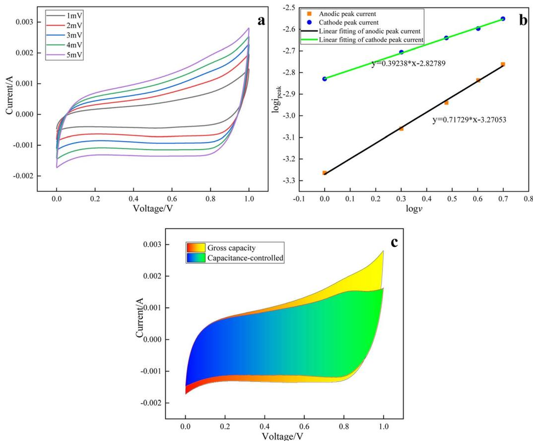
Fig. 9 Analysis diagram of the  $\gamma$ -MnO<sub>2</sub> electrode reaction process: (a) CV curves at different scanning speeds, (b) calculation of the  $b$  value, (c) calculation of the capacitance control area and total area.
