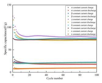
Fig. 13 Long charge-discharge cycles of electrode materials made of the five crystal forms of  $MnO_2$ .
