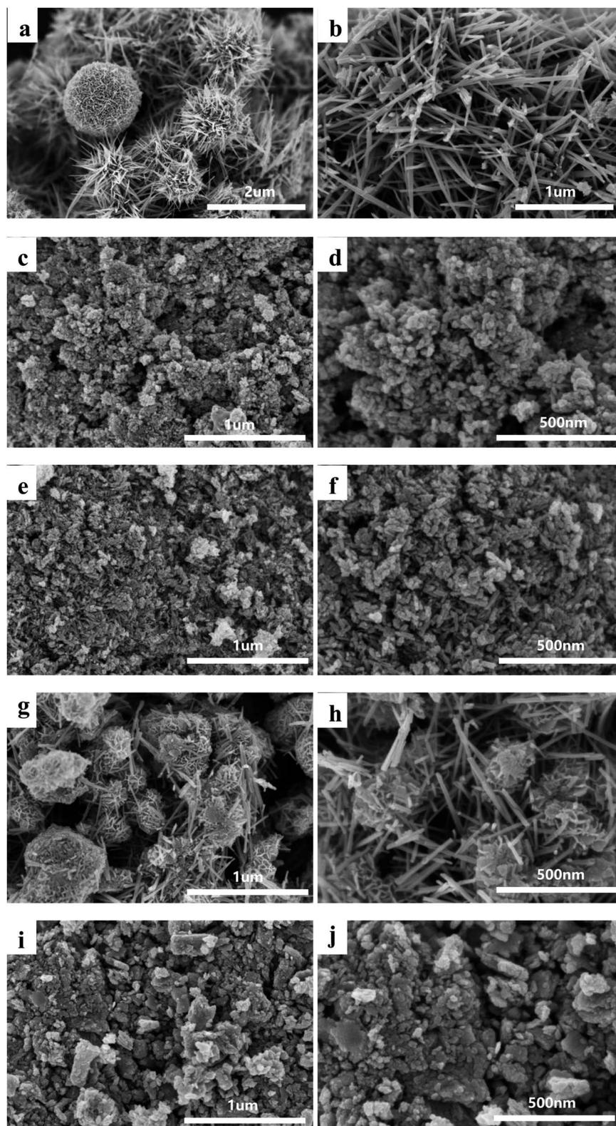
Fig. 2 SEM images of the different crystal forms of manganese dioxide: (a and b)  $\alpha$ - $\text{MnO}_2$ , (c and d)  $\beta$ - $\text{MnO}_2$ , (e and f)  $\gamma$ - $\text{MnO}_2$ , (g and h)  $\delta$ - $\text{MnO}_2$ , (i and j)  $\epsilon$ - $\text{MnO}_2$ .
