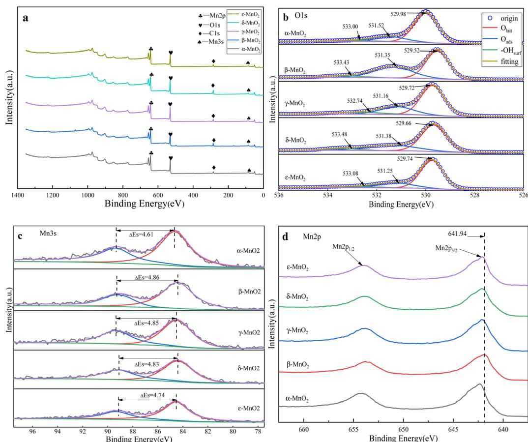
Fig. 4 XPS spectra of different crystal forms of manganese dioxide: (a) main spectrum, (b) O 1s spectrum, (c) Mn 3s spectrum, (d) Mn 2p spectrum.
