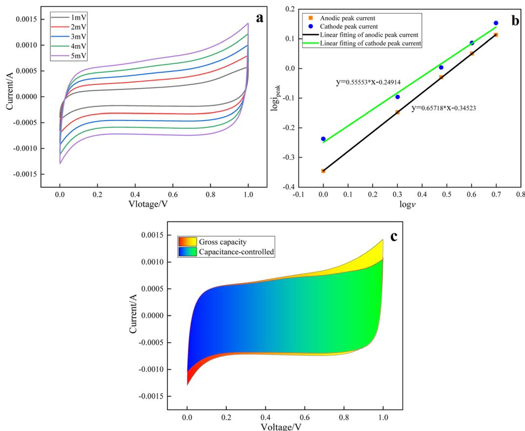
Fig. 8 Analysis diagram of the  $\beta\text{-MnO}_2$  electrode reaction process: (a) CV curves at different scanning speeds, (b) calculation of the  $b$  value, (c) calculation of the capacitance control area and total area.
