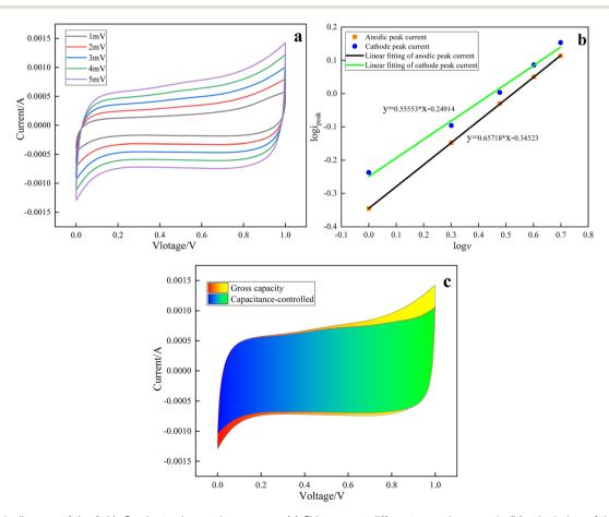
Fig. 8 Analysis diagram of the  $\beta$ -MnO<sub>2</sub> electrode reaction process: (a) CV curves at different scanning speeds, (b) calculation of the b value, (c) calculation of the capacitance control area and total area.
