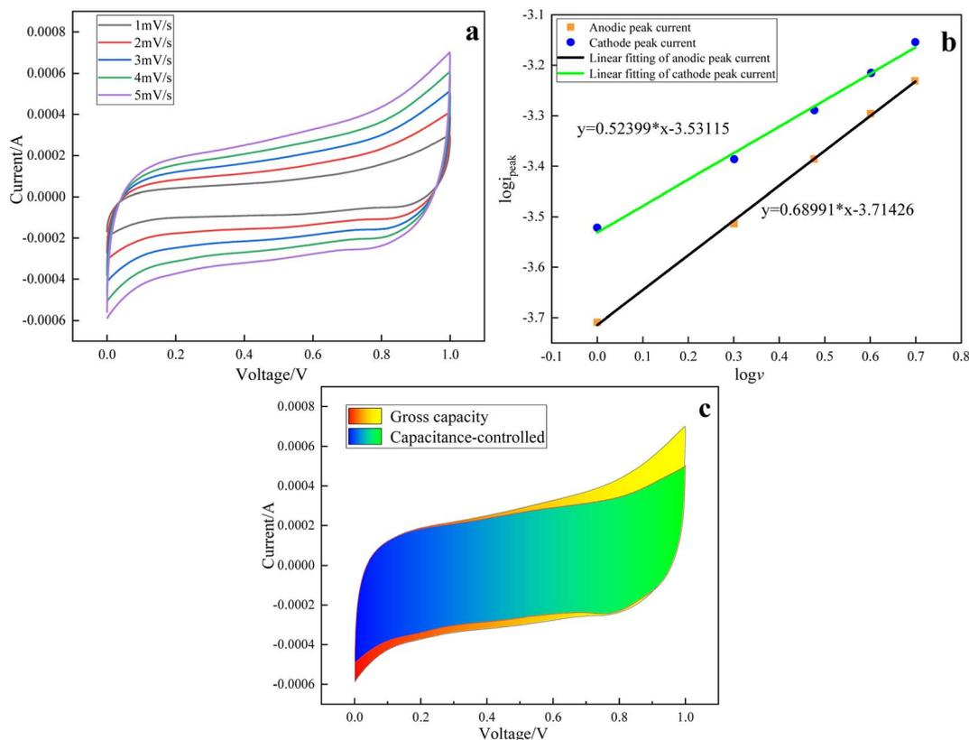
Fig. 7 Analysis diagram of the  $\alpha\text{-MnO}_2$  electrode reaction process: (a) CV curves at different scanning speeds, (b) calculation of the  $b$  value, (c) calculation of the capacitance control area and total area.
