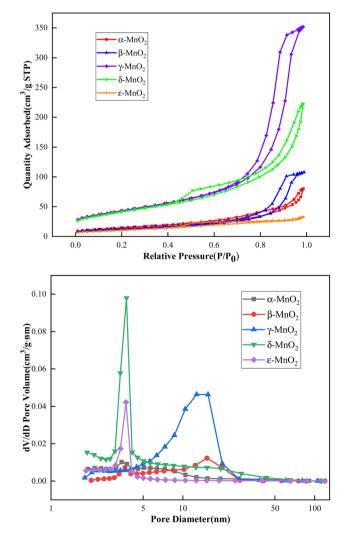
Fig. 3 Isothermal adsorption desorption and pore size distribution curves of different crystal forms of manganese dioxide.
