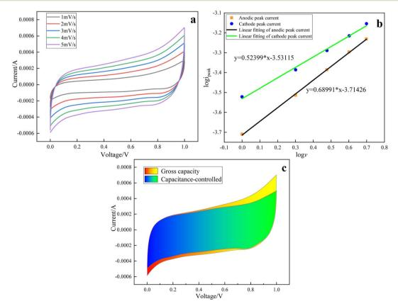
Fig. 7 Analysis diagram of the  $\alpha$ -MnO<sub>2</sub> electrode reaction process: (a) CV curves at different scanning speeds, (b) calculation of the *b* value, (c) calculation of the capacitance control area and total area.
