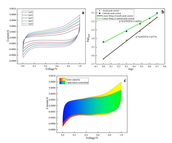
Fig. 11 Analysis diagram of the  $\epsilon$ -MnO<sub>2</sub> electrode reaction process: (a) CV curves at different scanning speeds, (b) calculation of the b value, (c) calculation of the capacitance control area and total area.
