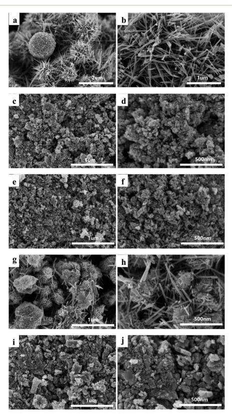
Fig. 2 SEM images of the different crystal forms of manganese dioxide: (a and b)  $\alpha$ -MnO<sub>2</sub>, (c and d)  $\beta$ -MnO<sub>2</sub>, (e and f)  $\gamma$ -MnO<sub>2</sub>, (g and h)  $\delta$ -MnO<sub>2</sub>, (i and j)  $\epsilon$ -MnO<sub>2</sub>.
