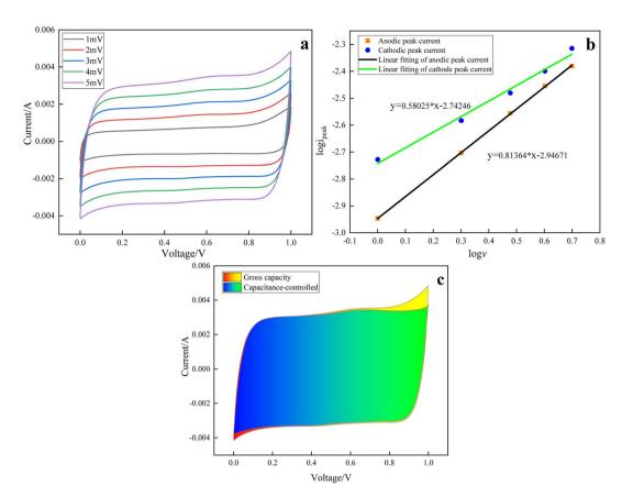
Fig. 10 Analysis diagram of the  $\delta$ -MnO<sub>2</sub> electrode reaction process: (a) CV curves at different scanning speeds, (b) calculation of the *b* value, (c) calculation of the capacitance control area and total area.
