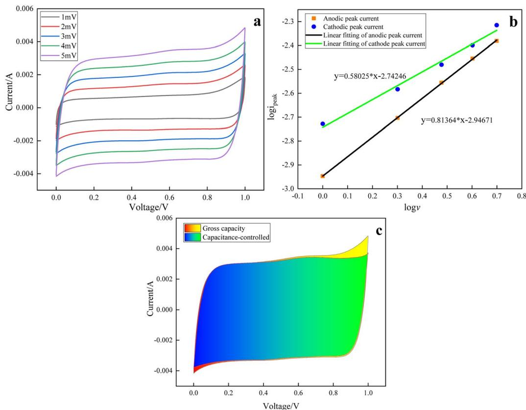
Fig. 10 Analysis diagram of the  $\delta$ -MnO<sub>2</sub> electrode reaction process: (a) CV curves at different scanning speeds, (b) calculation of the  $b$  value, (c) calculation of the capacitance control area and total area.
