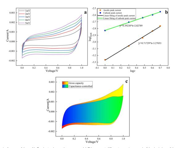
Fig. 9 Analysis diagram of the  $\gamma$ -MnO<sub>2</sub> electrode reaction process: (a) CV curves at different scanning speeds, (b) calculation of the *b* value, (c) calculation of the capacitance control area and total area.
