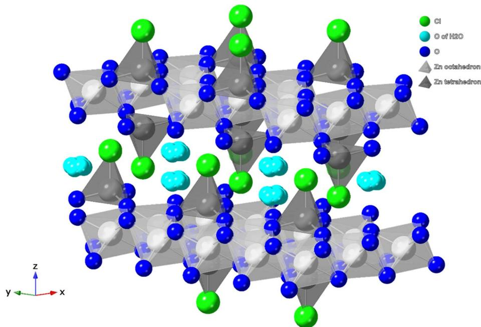
Fig. 1 The layered double hydroxide crystal structure of simonkolleite.<sup>15,60</sup> Zinc containing octahedron and tetrahedrons are shown (light and dark grey, respectively) with the interlayer spacing containing water. N. b. H atoms are not shown.
