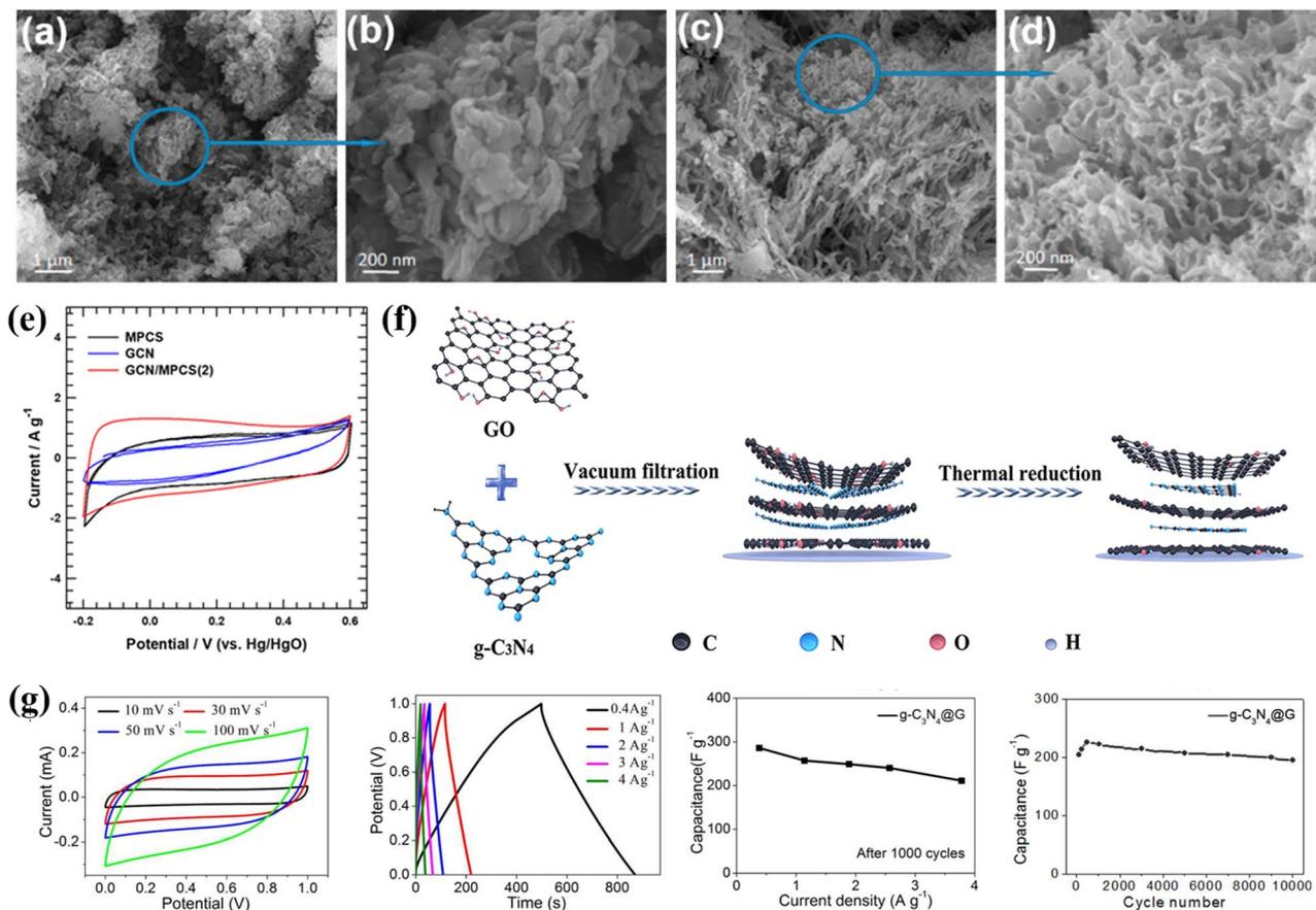
Fig. 8 (a–d) SEM images of BCN and TCN-200. (e) CV curves of pristine GCN, MPCs, and GCN/MPCS. (f) Schematic diagram of the synthesis of the graphene/g-C<sub>3</sub>N<sub>4</sub> composite, and (g) CV, GCD curves and corresponding capacitance value.
