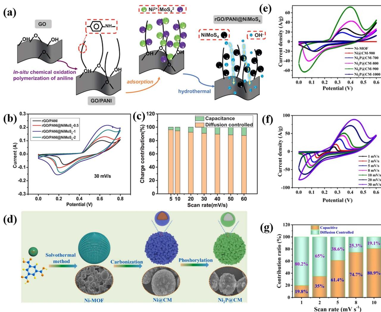
Fig. 4 (a) Preparation process schematic of rGO/PANI@NiMoS<sub>4</sub>, (b) CV curves at varying scan rates, (c) charge involvement of rGO/PANI@NiMoS<sub>4</sub>, (d) preparation process schematic of Ni<sub>2</sub>P@CM, a nanoscale nickel phosphide encapsulated in a carbon microsphere, (e) comparison of CV curves of composites, (f) CV curves of Ni<sub>2</sub>P@CM-900 at scan rates ranging from 1 mV s<sup>-1</sup> to 30 mV s<sup>-1</sup>, and (g) specific capacitance of composites.
