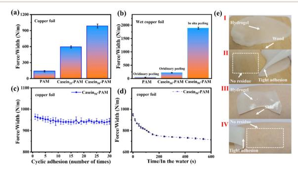
Fig. 7 (a) Comparison of peel strengths of PAM, casein<sub>25</sub>-PAM, and casein<sub>50</sub>-PAM hydrogel. (b) Comparison of peel strength between ordinary adhesion and the *in situ* polymerized CP hydrogel on wet copper foil. (c) Peeling strength of hydrogel during cyclic adhesion. (d) Peeling strength of the hydrogel soaked in water after adhesion. (e) Digital photos of the hydrogel adhering to wood/skin and peeling from wood/skin.
