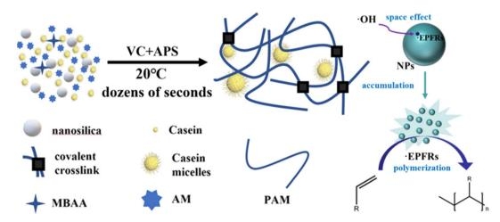
Scheme 1 Mechanism of fast polymerization based on a redox initiator system and persistent free radicals.
