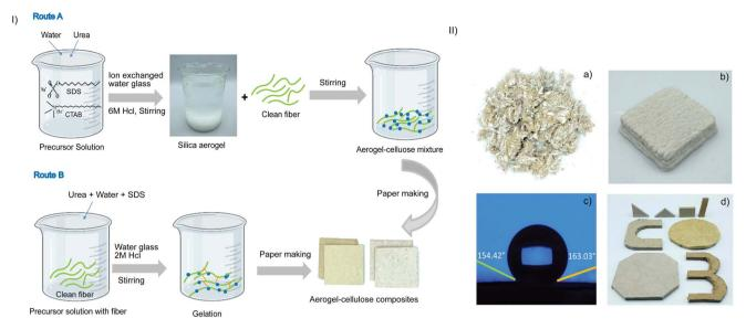
Fig. 1 (I) Schematic diagram of the *in situ* and physical mixing synthesis process of aerogel-cellulose composites, (II) (a) optical image of clean fiber, (b) 3D printing image of the composite, (c) image of the hydrophobic capability of the composite after trichlorosilane surface coating and (d) images showing different shapes and machinability of the aerogel-cellulose composite.
