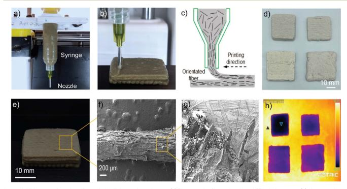
Fig. 4 Additive manufacturing of recycled cellulose pulp and paper. (a) Photograph of extrusion-based 3D printing setup, (b) close-up view at the nozzle region, (c) schematic diagram of fiber alignment during extrusion printing, (d) and (e) 3D-printed specimens with different thicknesses of the composites, (f) and (g) SEM images of 3D-printed composites, (h) thermal infrared (IR) image of the thermal insulation under 60 °C thermal heating
