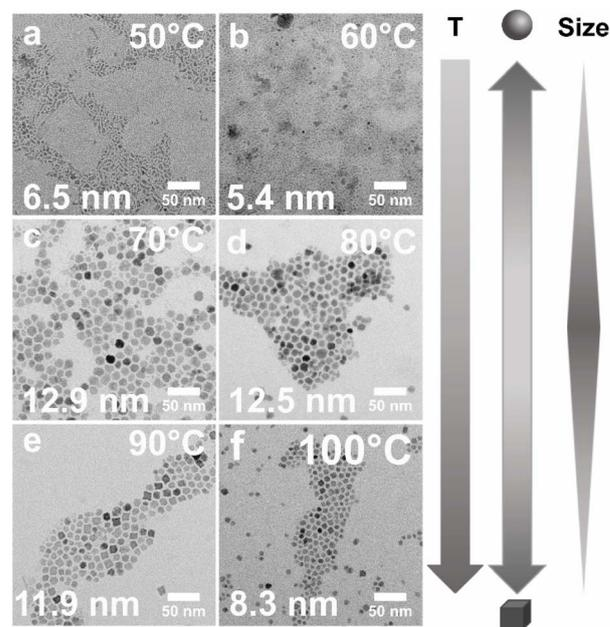
Fig. 2 Temperature-dependence of NP size and shape. TEM micrographs of  $\text{Co}_3\text{O}_4$  nanoparticles synthesized with a precipitation step performed at temperatures of (a) 50 °C, (b) 60 °C, (c) 70 °C, (d) 80 °C, (e) 90 °C and (f) 100 °C (same scale bar). Trends in the temperature-dependent modulation of particle size and shape are indicated by grey arrows.
