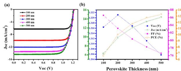
Fig. 4 Photovoltaic performance ( $J$ - $V$ ) (a) of the simulated Pb-free PSCs with the device architecture of FTO (500 nm)/TiO<sub>2</sub> (100 nm)/AgBi<sub>2</sub>I<sub>7</sub> (varying)/Spiro-MeOTAD (100 nm)/Au. Photovoltaic parameters (b) of the simulated Pb-free PSCs with the device architecture of FTO (500 nm)/TiO<sub>2</sub> (100 nm)/AgBi<sub>2</sub>I<sub>7</sub> (varying)/Spiro-MeOTAD (100 nm)/Au.
