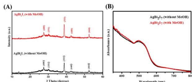
Fig. 1 PXRD peak pattern (A) and UV-vis absorption spectra (B) of AgBi<sub>2</sub>I<sub>7</sub> perovskite with MeOH (red) and without MeOH (black).
