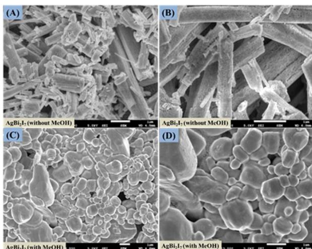
Fig. 2 FE-scanning electron microscopy images of AgBi<sub>2</sub>I<sub>7</sub> perovskite without MeOH (A and B) and with MeOH (C and D).
