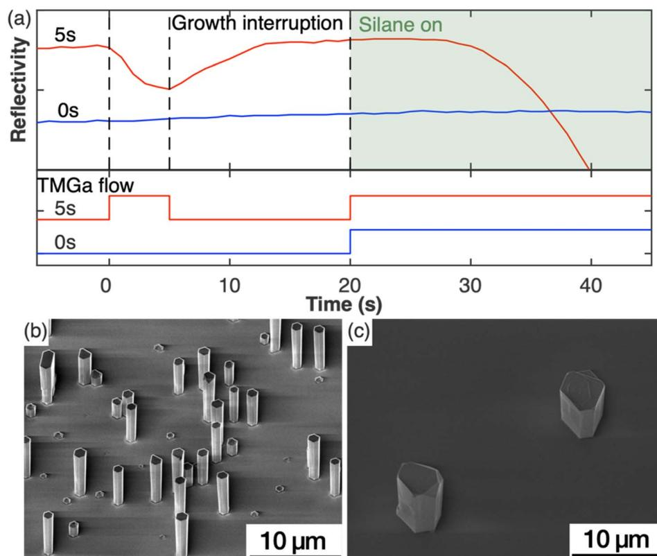
Fig. 1 (a) *In situ* reflectivity transients and the TMGa flow during the growth with (red) and without (blue) nucleation step. The shaded box highlights the introduction of silane flow. (b and c) SE images of GaN nanowires grown with (5 s) and without (0 s) nucleation step.
