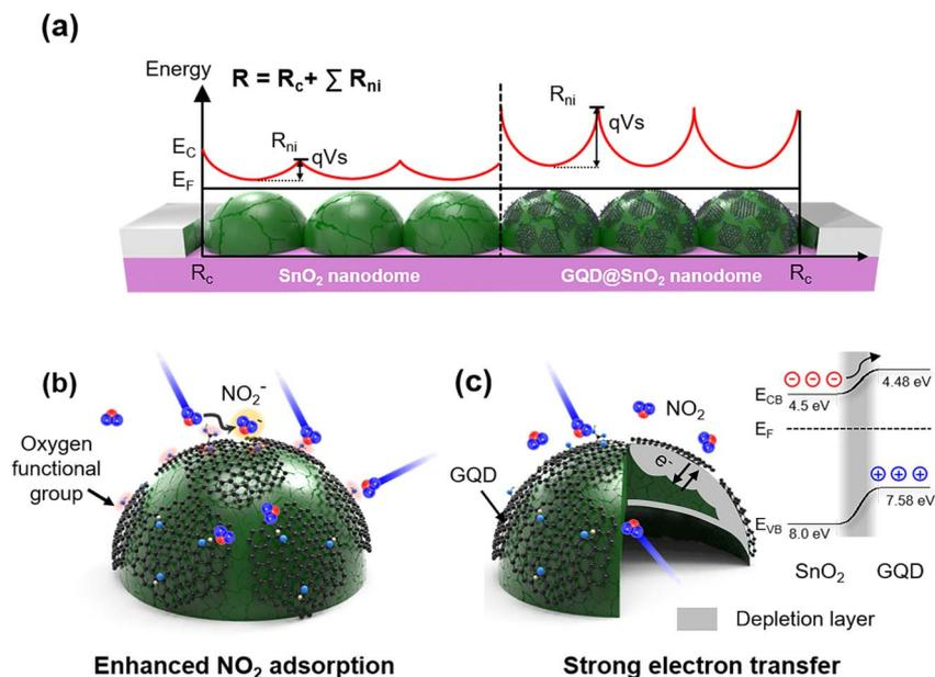
Fig. 5 Schematic illustration for (A) initial potential barrier formation for the SnO<sub>2</sub> nanodomains structure. (B and C) Schematic illustration of the NO<sub>2</sub> sensing mechanism for GQD@SnO<sub>2</sub> nanodomains showing (B) enhanced NO<sub>2</sub> adsorption due to the GQDs and (C) formation of an electron depletion layer with its electronic band structure.
