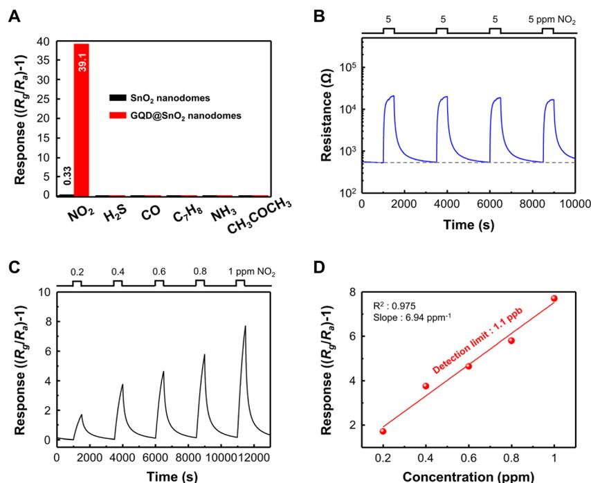
Fig. 3 (A) Selective NO<sub>2</sub> gas sensing performance of GQD@SnO<sub>2</sub> nanodome based gas sensors. (B) Resistance curve of GQD@SnO<sub>2</sub> to 5 ppm NO<sub>2</sub> with repeated exposure. (C) Response curves to different NO<sub>2</sub> concentrations under a 1 ppm concentration. (D) Linear fit of the responses as a function of NO<sub>2</sub> concentration.
