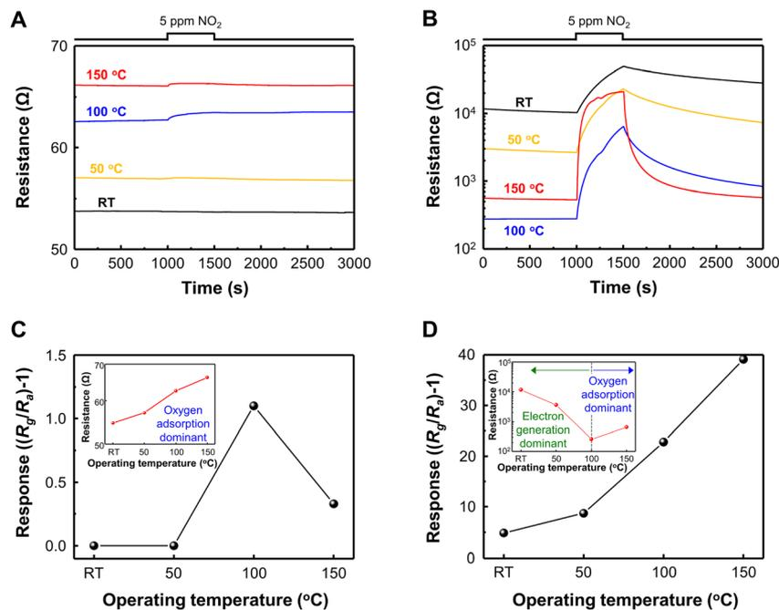
Fig. 2 Resistance curves for 5 ppm NO<sub>2</sub> as a function of operating temperature for (A) pristine SnO<sub>2</sub> nanodomains and (B) a GQD@SnO<sub>2</sub> nanodome based gas sensor. Gas response for (C) pristine SnO<sub>2</sub> nanodomains and (D) a GQD@SnO<sub>2</sub> nanodome based gas sensor. The insets of (C and D) represent the base resistance as a function of operating temperature.
