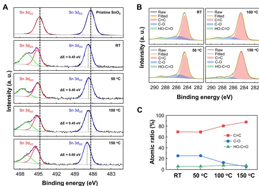
Fig. 4 X-ray photoelectron spectroscopy (XPS) (A) Sn 3d and (B) C 1s spectra of pristine SnO<sub>2</sub> nanodomains and GQD@SnO<sub>2</sub> nanodomains prepared at various annealing temperatures. (C) Atomic ratio of carbon bonds as a function of annealing temperature.
