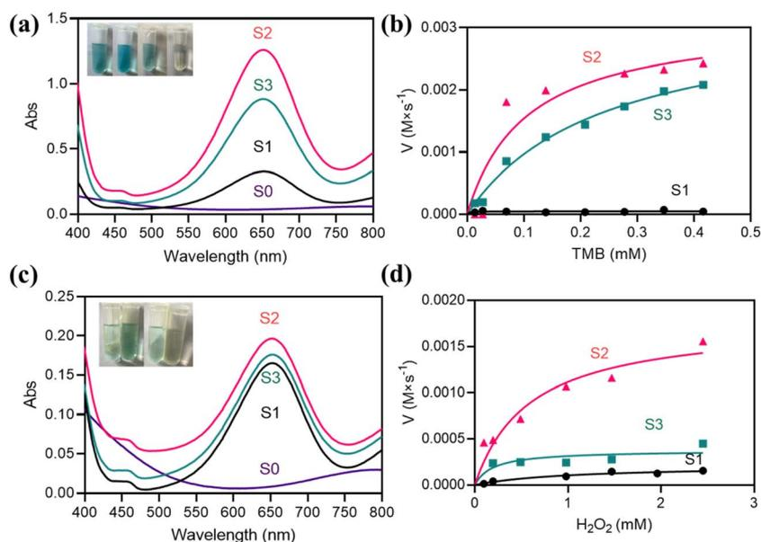
Fig. 2 (a) UV absorption spectra of TMB + S0, TMB + S1, TMB + S2 and TMB + S3; (b) concentration versus the reaction rate for TMB as a substrate; (c) UV absorption spectra of TMB + H<sub>2</sub>O<sub>2</sub> + S0, TMB + H<sub>2</sub>O<sub>2</sub> + S1, TMB + H<sub>2</sub>O<sub>2</sub> + S2 and TMB + H<sub>2</sub>O<sub>2</sub> + S3; (d) concentration versus the reaction rate for H<sub>2</sub>O<sub>2</sub> as a substrate.
