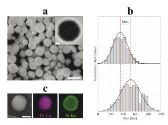
Fig. 5 SEM micrograph (a) of SiO $_2$ -Lys-SP-NCs. Scale bar of 1  $\mu$ m. In the inset, TEM micrograph of a single-NC with a scale bar of 100 nm. Dry size distribution and Gaussian fit comparison (b) between uncoated (top,  $R^2=98\%$ ) and coated (bottom,  $R^2=88\%$ ) SP-NCs, highlighting the (double) shell thickness (170 nm). EDX mapping (c) of a single SiO $_2$ -Lys-SP-NC, detecting Fe L $\alpha$  and Si K $\alpha$  characteristic X-ray emission lines. Scale bar indicates 250 nm.
