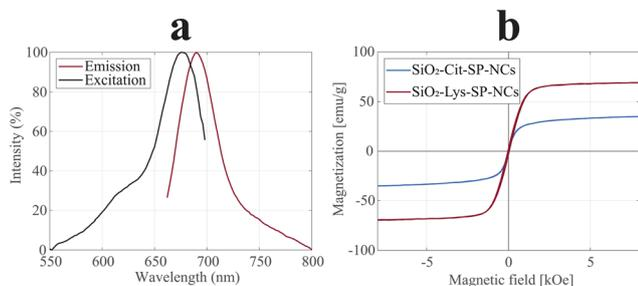
**Fig. 6** PL spectra (a) of SiO<sub>2</sub>-Lys-SP-NCs, with excitation (black) and emission (red) plots, highlighting excitation maximum at 675 nm and emission maximum at 690 nm. Magnetization curves (b) of SiO<sub>2</sub>-Cit-SP-NCs (blue) and SiO<sub>2</sub>-Lys-SP-NCs (red), normalized to the inorganic content.
