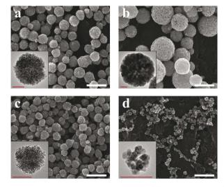
Fig. 1 SEM micrographs of the synthesized (a) Cit-SP-NCs (ST), (b) Lys-SP-NCs (ST), (c) Cit-SP-NCs (MW), (d) Lys-SP-NCs (MW). Scale bars indicate 500 nm (in white). In the insets, TEM micrographs of single SP-NCs for the primary particle size estimation. Scale bars in the insets indicate 100 nm (in red).
