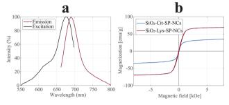
Fig. 6 PL spectra (a) of SiO<sub>2</sub>-Lys-SP-NCs, with excitation (black) and emission (red) plots, highlighting excitation maximum at 675 nm and emission maximum at 690 nm. Magnetization curves (b) of SiO<sub>2</sub>-Cit-SP-NCs (blue) and SiO<sub>2</sub>-Lys-SP-NCs (red), normalized to the inorganic
