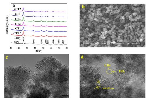
Fig. 1 XRD patterns of TiO<sub>2</sub> NPs and CDs/TiO<sub>2</sub> (a), SEM (b), and HRTEM images (c and d) of CT2.
