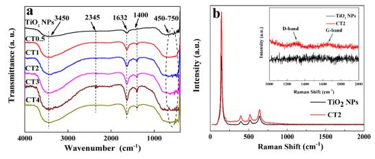
Fig. 3 FT-IR spectra of TiO<sub>2</sub> NPs and CDs/TiO<sub>2</sub> (a), and Raman spectra of TiO<sub>2</sub> NPs and CT2 (b).
