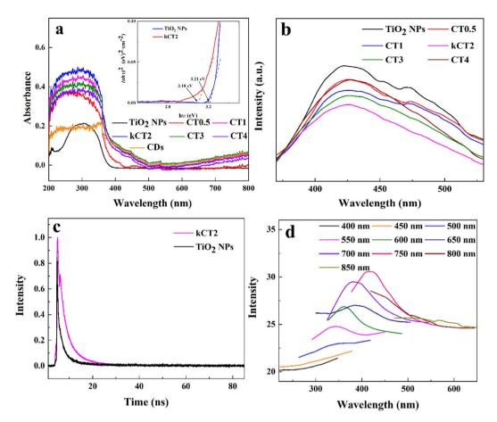
Fig. 7 UV-vis spectra of TiO<sub>2</sub> NPs and CDs/TiO<sub>2</sub> (a) and Tauc plots (inset) of TiO<sub>2</sub> NPs and kCT2, PL spectra of TiO<sub>2</sub> NPs and CDs/TiO<sub>2</sub> (b), TRPL spectra of TiO<sub>2</sub> NPs and kCT2 (c), and up-converted PL spectra of gCDs at different excitation wavelengths (d).
