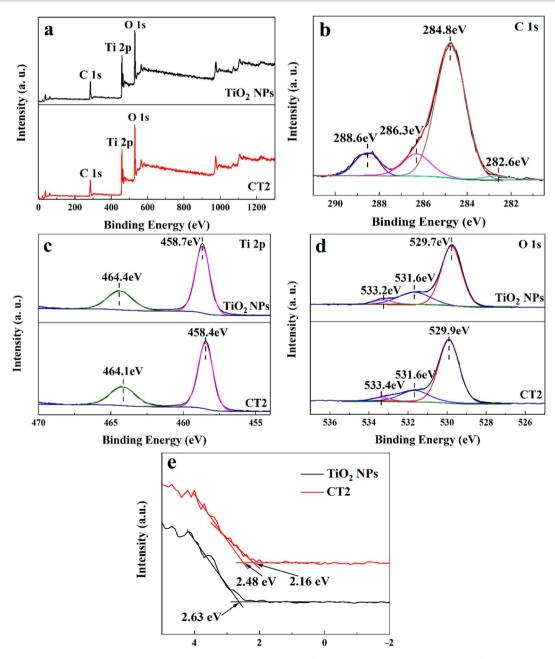
Fig. 4 XPS survey spectra (a), the corresponding high-resolution XPS spectra (b-d) of C 1s (b), Ti 2p (c) and O 1s (d), and VB-XPS spectra (e) of TiO<sub>2</sub> NPs and CT2.
