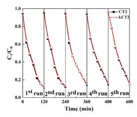
Fig. 6 Five consecutive cycles of photocatalytic degradation of MO over CT2 and kCT2.
