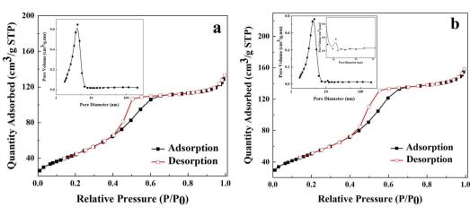
Fig. 2 N<sub>2</sub> adsorption-desorption curves and pore size distribution (inset) of TiO<sub>2</sub> NPs (a) and kCT2 (b).
