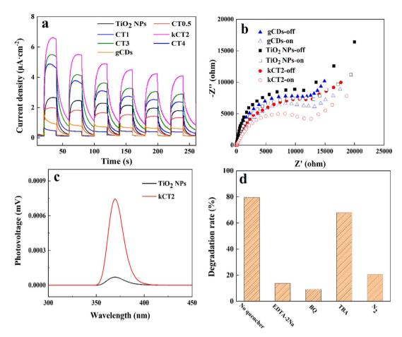
Fig. 8 Transient photocurrent responses of various samples (a), EIS plots of  $TiO_2$  NPs, gCDs and kCT2 with and without light (b), SPV curves of  $TiO_2$  NPs and kCT2 (c), and trapping experiments of active species for the MO removal over kCT2 under irradiation (d).
