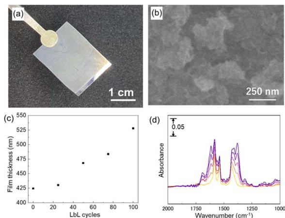
**Fig. 3** (a) A photo and (b) an SEM image of a  $\text{Cu}_2(\text{BPYDC})_2$ -on- $\text{Cu}_2(\text{BPDC})_2$  thin film synthesized after 50 LbL cycles. (c) Total thickness and (d) FT-IR spectra of the  $\text{Cu}_2(\text{BPYDC})_2$ -on- $\text{Cu}_2(\text{BPDC})_2$  thin film as a function of LbL cycles. The thickness is measured with a stylus profilometer.
