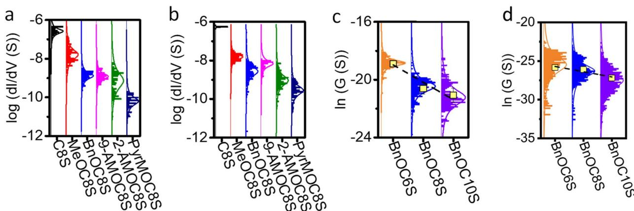
**Fig. 2** Experimental results for the electrical conductances of different SAMs. Conductance distribution of SAMs obtained using (a) a Pt coated probe and (b) a graphene coated probe. The distribution of conductances *versus* the number of alkyl units, obtained using (c) a Pt coated probe and (d) a graphene coated probe for molecules with a benzyl head group (average conductance is indicated by the yellow squares).
