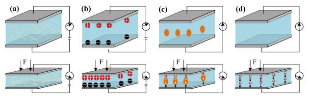
Fig. 2 Sensing mechanisms of the pressure sensors. (a) Piezoresistive type; (b) capacitive type; (c) piezoelectric type; (d) triboelectric type.
