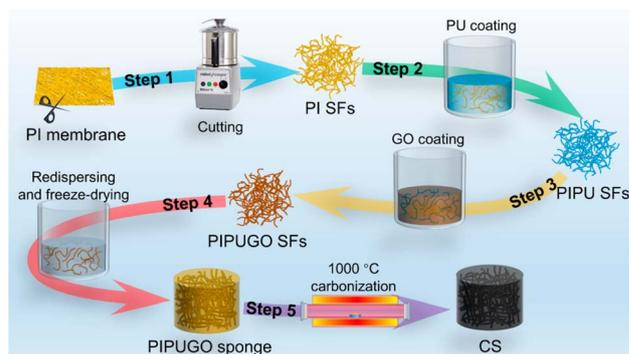
Fig. 3 The fabrication procedure of carbon fibrous sponges.<sup>132</sup> Reproduced with permission. Figure has been adapted/reproduced from ref. 132 with permission from American Chemical Society, copyright 2022.
