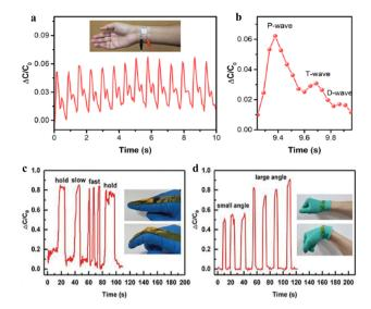
Fig. 5 The main application of capacitive sensors, (a) and (b) are pulse wave monitoring:141 (c) and (d) are finger and wrist bending.142 Reproduced with permission. Figure (a and b) has been adapted/ reproduced from ref. 141 with permission from American Chemical Society, copyright 2020. Figure (c and d) has been adapted/reproduced from ref. 142 with permission from Wiley-VCH GmbH, copyright 2021.
