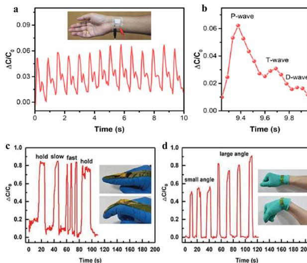
Fig. 5 The main application of capacitive sensors, (a) and (b) are pulse wave monitoring;<sup>141</sup> (c) and (d) are finger and wrist bending.<sup>142</sup> Reproduced with permission. Figure (a and b) has been adapted/reproduced from ref. 141 with permission from American Chemical Society, copyright 2020. Figure (c and d) has been adapted/reproduced from ref. 142 with permission from Wiley-VCH GmbH, copyright 2021.
