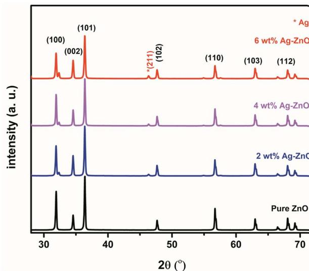
Fig. 3 XRD patterns of pure and Ag-doped ZnO NPs.
