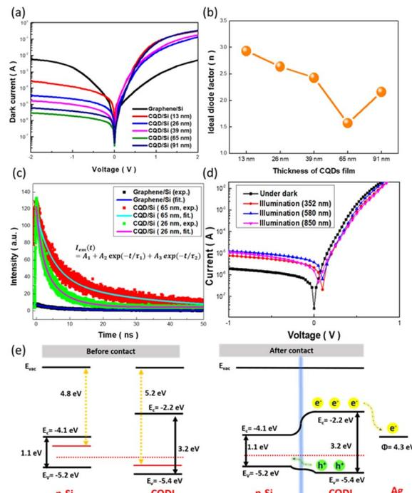
Fig. 4 (a) Dark  $I$ - $V$  curves of various CQDL/Si and graphene/Si-based devices. (b) Extracted ideal diode factor with respect to the thickness of the CQDL. (c) TRPL examinations of graphene/Si, CQDL (26 nm)/Si and CQDL (65 nm)/Si. The correlated exponential fittings are also shown. (d) Light-driven  $I$ - $V$  results of CQDL (65 nm)/Si under various light illuminations. (e) Schematic presentation of band diagrams before and after CQDLs coming into contact with Si substrates.
