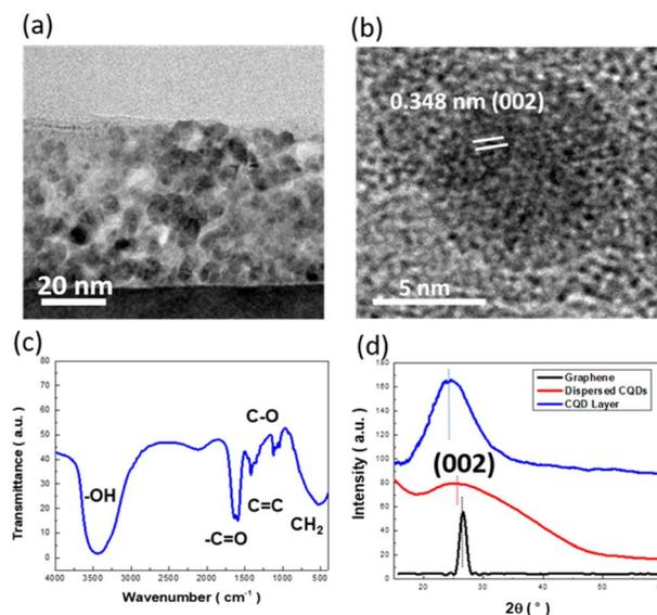
Fig. 1 (a) Cross-sectional TEM image of CQDL directly formed on Si substrate. (b) HRTEM image of a representative CQD. (c) FTIR results of CQDL with a thickness of  $65 \text{ nm}$ . (d) XRD patterns of graphene, dispersed CQDs and CQDL.
