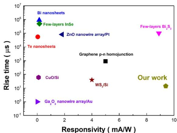
Fig. 7 Comparison of device performance of broadband photodetectors in terms of rise time and specific responsivity.
