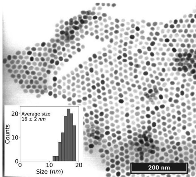
Fig. 3 The STEM image acquired in the transmission mode shows the UCNPs with an average size of  $16 \pm 2$  nm and hexagonal morphology. The inset displays their size distribution histogram taken from 100 nanoparticles.
