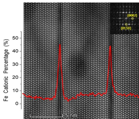
Fig. 4 STEM-HAADF image of the IDB sample along the ZnO-[ $\bar{2}110$ ] projection. The inset shows the corresponding FFT. The EDS profile of Fe in cationic percentage is superimposed on the HAADF image. The EDS signal was collected from the entirety of the displayed area, and the Fe-signal was averaged vertically to produce the superposed line profile.
