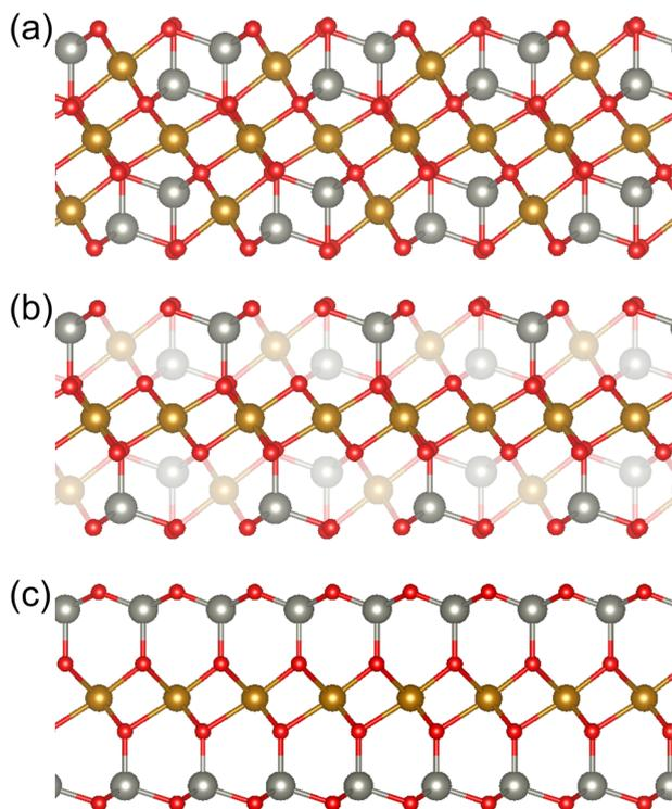
Fig. 5 Comparison of atomic structure of (a) a layer of Fe atoms octahedrally coordinated by O on a {111} plane in ZnFe<sub>2</sub>O<sub>4</sub> (projection [101]), and (c) schematic representation of an Fe-decorated b-IDB in ZnO (projection [11 $\bar{2}$ 0]). In (b) the similarities in the two structures are highlighted by making some of the atoms in the ZnFe<sub>2</sub>O<sub>4</sub> structure transparent. Atoms are shown in gray (Zn), red (O) and gold (Fe).
