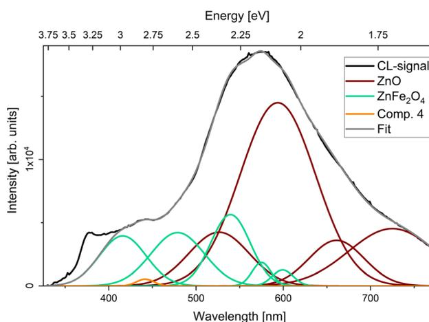
Fig. 9 CL spectrum acquired at 80 K from the IDB sample. The spectral deconvolution using emission components from bulk ZnO and bulk  $\text{ZnFe}_2\text{O}_4$  is shown. A final component was added at 2.8 eV (orange line).
