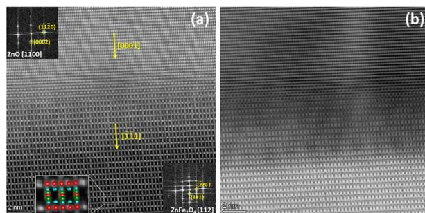
Fig. 3 High resolution (a) STEM-HAADF and (b) STEM-ABF images of the interface between a ZnFe<sub>2</sub>O<sub>4</sub> NP and the ZnO matrix in the nanocomposite sample. Insets show FFTs from the corresponding areas and a schematic representation of the atomic structure of ZnFe<sub>2</sub>O<sub>4</sub> overlaid on the magnified HAADF image from the ZnFe<sub>2</sub>O<sub>4</sub> particle (Zn in green, Fe in red, and O in blue). Yellow arrows indicate the directions of the lattice matching.
