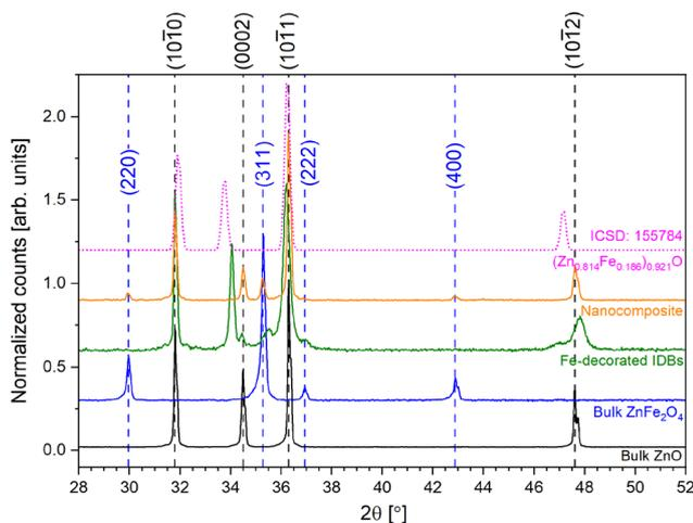
Fig. 1 Diffractograms from all samples in Table 1. A zero-point shift has been applied. Peak positions for ZnFe<sub>2</sub>O<sub>4</sub> and ZnO have been indicated by dotted lines and indices (blue for ZnFe<sub>2</sub>O<sub>4</sub>, black for ZnO). The pink dotted line shows the diffractogram from an Fe-rich ZnO solid solution obtained from ICSD (ICSD: 155784).
