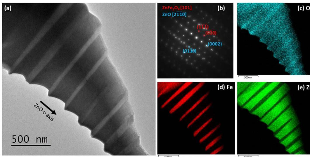
Fig. 2 (a) Bright field STEM image from the nanocomposite sample, taken along the ZnO-[ $\bar{2}110$ ]-projection. (b) Indexed SAED pattern from a large part of the area in (a), showing diffraction from both the ZnO matrix and the ZnFe<sub>2</sub>O<sub>4</sub> NPs. (c)–(e) STEM EDS maps showing an accumulation of Fe and a depletion of Zn at the ZnFe<sub>2</sub>O<sub>4</sub> NPs, compared to the ZnO matrix.
