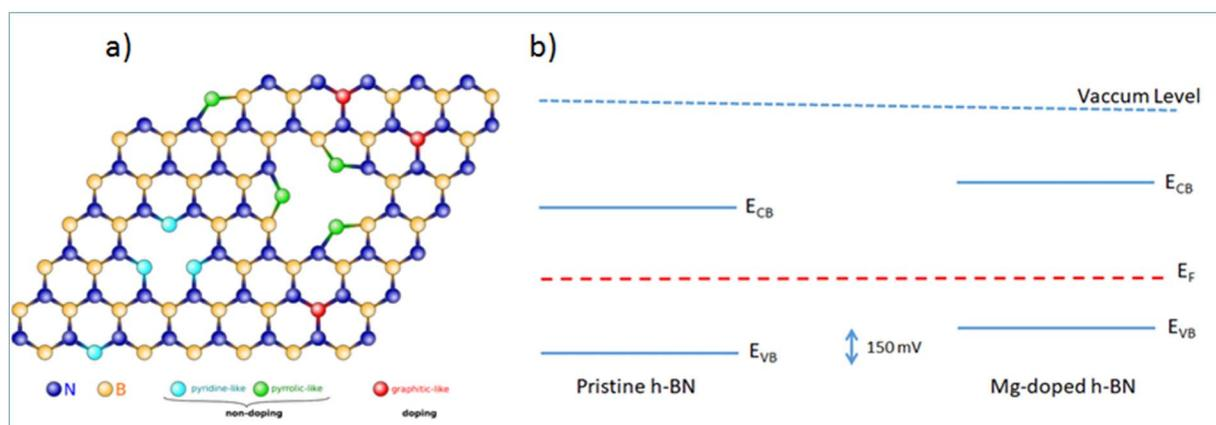
Fig. 5 (a) Proposed atomic arrangements of Mg impurities in h-BN of the three suggested Mg incorporation sites: graphitic, pyrrolic, and pyridinic. The crystal is viewed along the *c*-axis. (b) Band alignment and offset in our h-BN/graphene heterostructures, as determined from the ARPES data.
