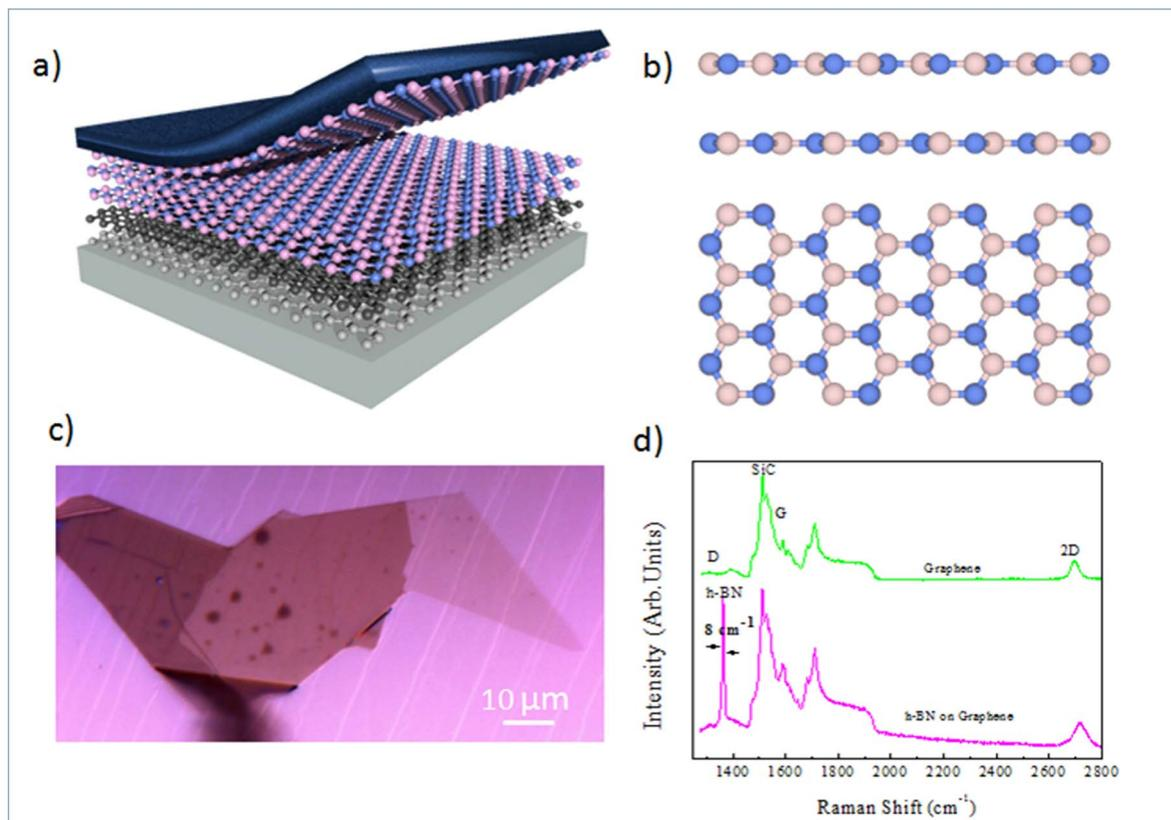
**Fig. 1** Crystal structure and micro-Raman spectroscopy of multilayer Mg doped h-BN: (a) graphical representation of the mechanical exfoliation of the h-BN sample on the graphene/SiC surface. (b) Crystal structure of the 2H (AA') h-BN polytype. (c) Optical image of the Mg-doped h-BN sample, as exfoliated on graphene/SiC surface. (d) Micro-Raman spectra of h-BN/graphene and reference graphene area (532 nm laser, room temperature).
