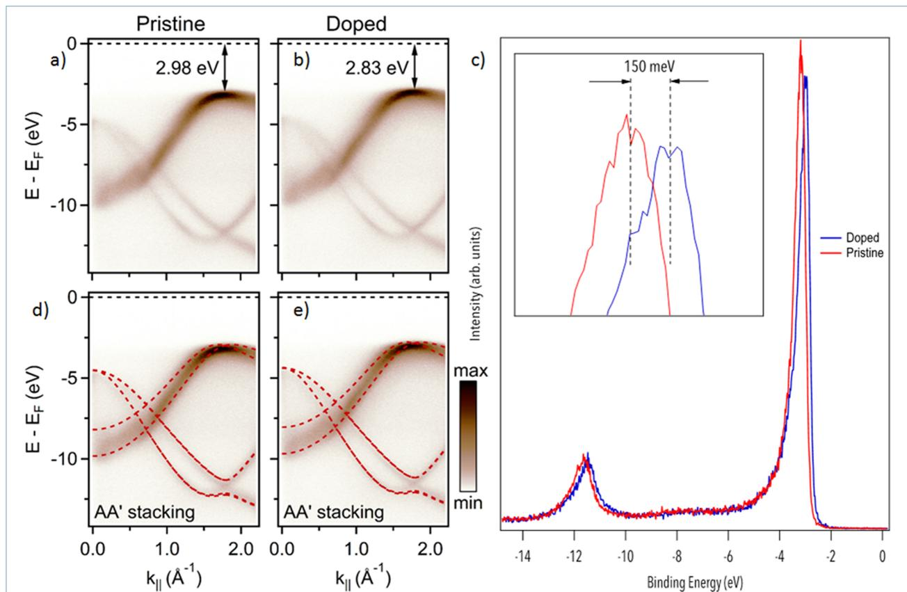
Fig. 3 Electronic structure of pristine and Mg doped h-BN: (a and b) nano-ARPES spectra of pristine h-BN and Mg-doped h-BN acquired at photon energy  $h\nu = 100$  eV, respectively. (c) Nano-ARPES intensity integrated spectra as a function of the binding energy, extracted from the 2D ARPES map, for pristine h-BN (red line) and Mg-doped h-BN (blue line). (d and e) Same nano-ARPES data with superposed band structure from DFT calculation (PBE) of bulk hexagonal AA' h-BN.
