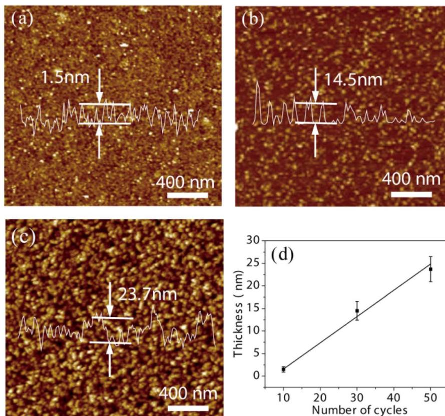
Fig. 2 AFM images of NbS<sub>2</sub> films obtained by 10 (a), 30 (b), and 50 (c) ALD cycles. (d) Thickness of the NbS<sub>2</sub> film against the number of ALD cycles.
