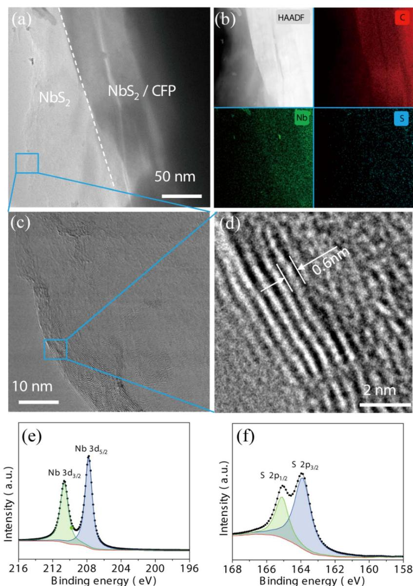
Fig. 4 (a) TEM image of NbS<sub>2</sub>NFs/CFP. (b) High-angle annular dark-field (HAADF) images of the area in (a) and its elemental mapping images of C, Nb, and S, respectively. (c and d) HRTEM images of the local area in (a). XPS spectra of Nb 4f (e) and S 2p (f).
