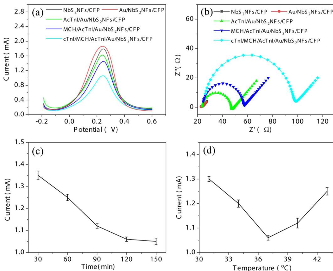
Fig. 6 (a) DPV and (b) EIS curves of different modifiers based on NbS<sub>2</sub>NFs/CFP. The equivalent circuit is shown in Fig. S2.† Influence of the hybridization time (c) and temperature (d) on peak current ( $n = 3$ ).
