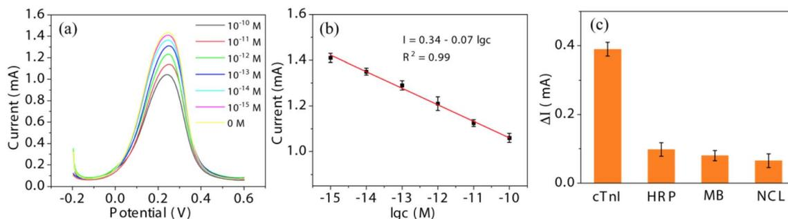
Fig. 7 (a) DPV response of the biosensor to various concentrations of cTnI (from 0 to  $10^{-10}$  M). (b) The response current of (a) as a function of logarithm of concentration ( $n = 3$ ). (c) Comparison of cTnI response current with other proteins (HRP, MB and NCL), indicating the excellent selectivity of the fabricated biosensor.
