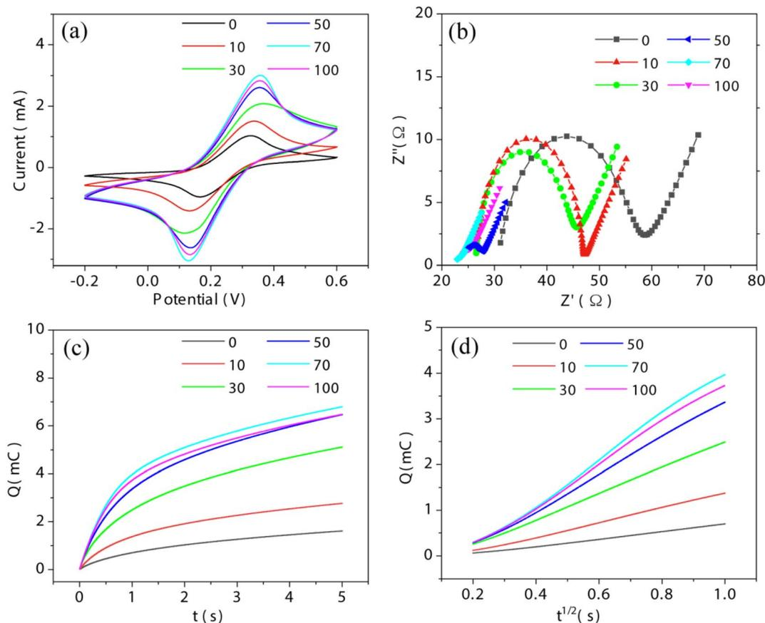
Fig. 5 (a) CV, (b) EIS, (c)  $Q-t$ , and (d)  $Q-t^{1/2}$  curves of bare CFP and  $\text{NbS}_2\text{NFs}/\text{CFP}$  obtained by different ALD cycles. 0, 10, 30, 50, 70 and 100 are bare CFP, 10, 30, 50, 70 and 100 ALD cycles respectively.
