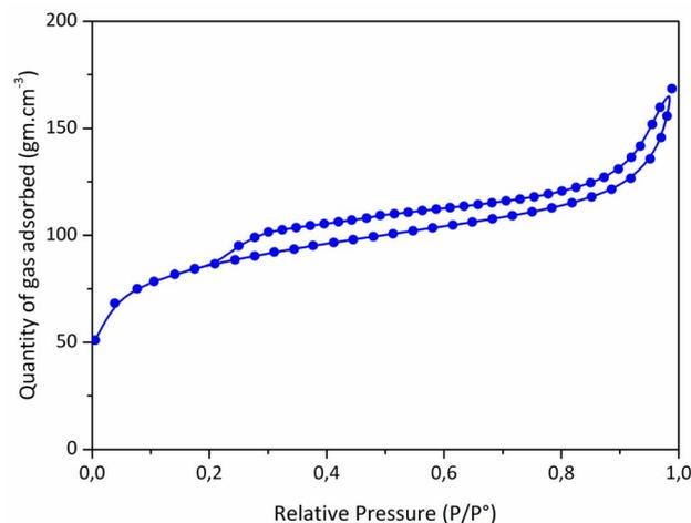
Fig. 3  $\text{N}_2$  sorption isotherms of the PSZNi2.5\_5 sample.
