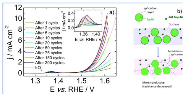
Fig. 7 (a) Polarization curves recorded at  $5 \text{ mV s}^{-1}$  after different numbers of voltammetric cycles in nitrogen saturated 1 M KOH electrolyte, (b) schematic showing removal of the carbon shell surrounding fcc-Ni particles to be redistributed within the Si–C–O–N(H) matrix under working conditions in a 1 M KOH electrolyte.
