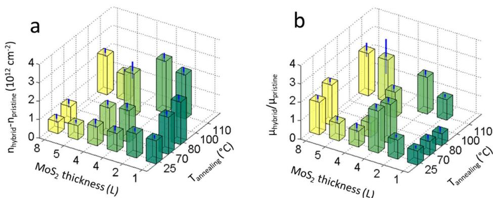
Fig. 5 Annealing temperature dependence of the induced doping (a) and the field effect mobility (b) measured on six samples of MoS<sub>2</sub> thicknesses 1L, 2L, 4L, 4L, 5L and 8L.
