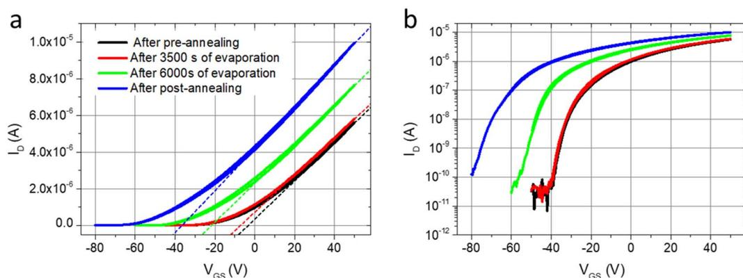
**Fig. 4** (a) Transfer characteristic recorded at  $V_{DS} = 1 \text{ V}$  of the device annealed *in situ* (black), after the first molecular deposition (red), after the second molecular deposition (green) and after the post-annealing (blue). Both gate voltage sweep directions are plotted, which shows negligible hysteresis. (b) Same transfer characteristics presented in semi-log scale.
