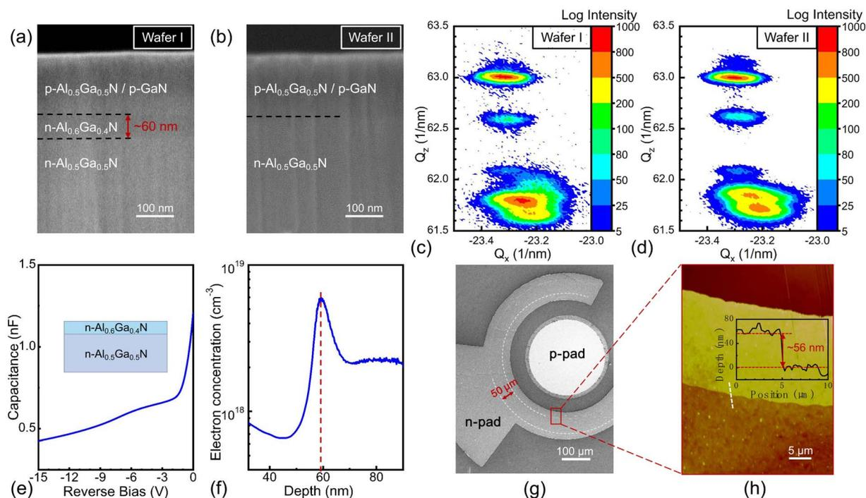
Fig. 2 (a) and (b) are the cross-sectional SEM images of Wafer I and II. (c) and (d) are the XRD RSMs of the  $(-105)$  plane of Wafer I and II. (e) and (f) are the  $C-V$  measurement result and the depth-dependent electron concentration profile of the  $\text{Al}_{0.5}\text{Ga}_{0.5}\text{N}/\text{Al}_{0.6}\text{Ga}_{0.4}\text{N}$  wafer. (g) Top-view SEM image of the fabricated Device A. (h) AFM image of the selected region in (g). The inset is the depth profile of recess edge.
