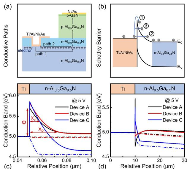
Fig. 5 (a) Electron transport path diagram in Device A. (b) Electron transport processes at the MS contact.  $E_C$  and  $E_V$  represent the conduction and the valence bands, respectively. (c) and (d) are the calculated conduction band diagrams of metal/n-AlGa<sub>0.5</sub>N contact along paths 1 and 2 in Devices A, B and C at 5 V, respectively.
