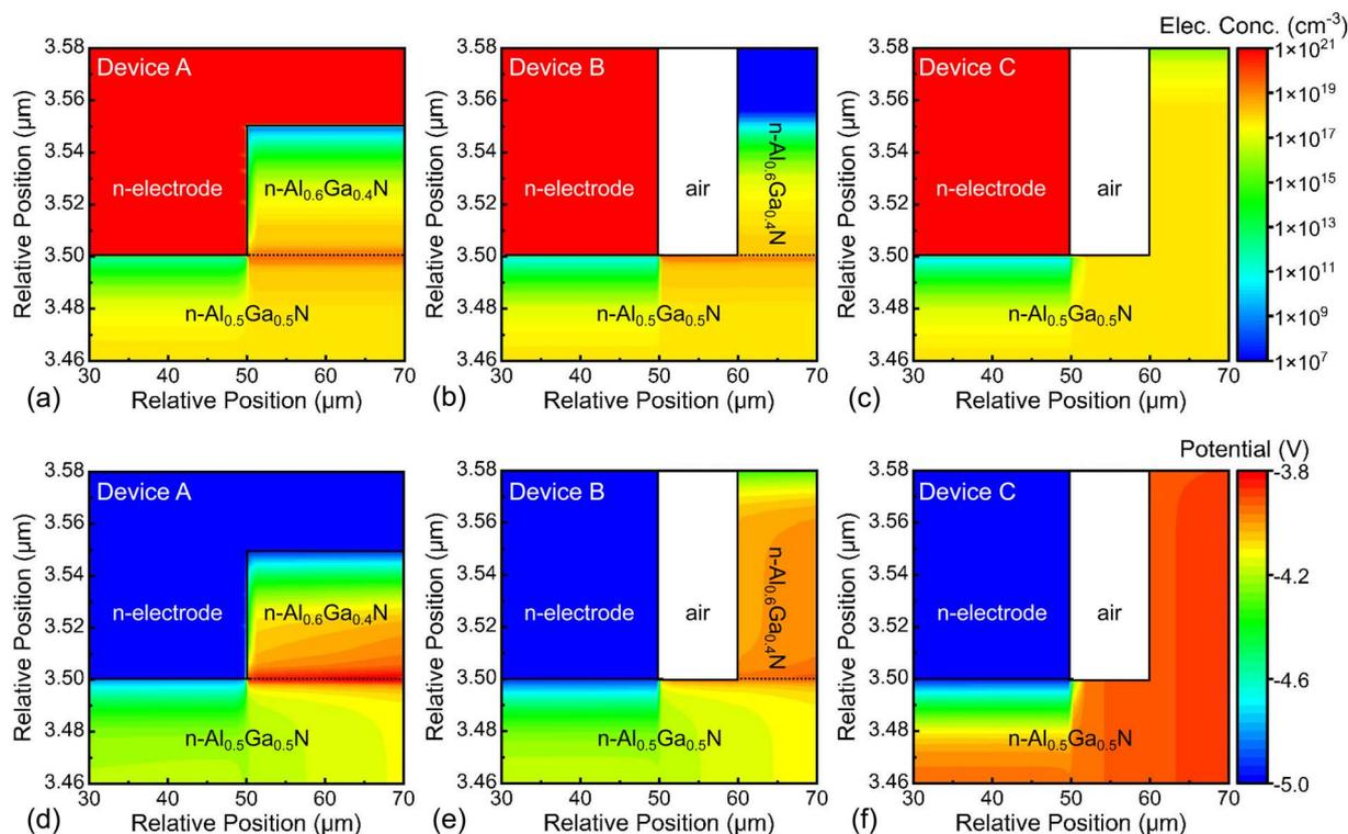
Fig. 4 (a)–(c) Local electron concentration distribution at equilibrium and (d)–(f) potential distributions at 5 V near n-contact in Devices A, B and C.
