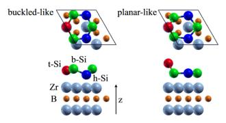
Fig. 8 Structures of buckled-like and planar-like silicene, where the top Si (red), bridge Si (green), and hollow Si (blue) are indicated. Adapted with permission from ref. 150, Copyright 2017 by the American Physical Society.
