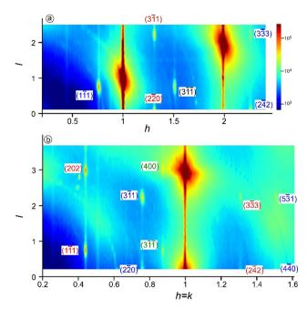
Fig. 9 Maps of the intensity diffracted by 8 ML of Si evaporated on Ag(111) at 520 K growth. The h, k indices correspond to in-plane directions, whereas l corresponds to the out-of-plane direction. (a) Map for k=0. (b) Map for h=k. The color scale is the same for both maps. The indexed spots belong to diamond-like silicon with four orientations (corresponding to blue, red, green and black labels). Reprinted with permission of IOP Publishing, Ltd, from ref. 165, Copyright 2017.
