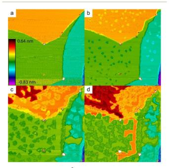
Fig. 2 STM images (325 nm)<sup>2</sup> of the evolution of the Ag(111) surface during Si evaporation at 440 K. (a) Bare surface. (b–d) For Si coverages of 0.09, 0.49 and 0.74 ML, respectively. Triangular domains correspond to inserted silicene islands, while outgrowths forming from the terraces correspond to Ag expelled atoms that recondense. Adapted from ref. 86, with permission of AIP Publishing.
