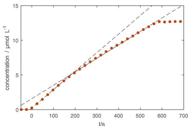
**Fig. 4** Total concentration of Si determined through fitting the four Si–O–Si stretching modes in the IR spectrum. The growth rate changes after about 150 seconds from  $0.23 \mu\text{mol L}^{-1} \text{s}^{-1}$  to  $0.17 \mu\text{mol L}^{-1} \text{s}^{-1}$  and is indicated with dashed lines.
