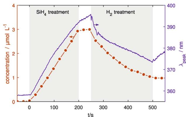
Fig. 6 Deposition and etching experiment with SiO<sub>2</sub> coated Ag NPs. Ag NPs were injected into the treatment chamber, coated using SiH<sub>4</sub> and subsequently etched using H<sub>2</sub> (both marked in grey). This procedure was done once with UV-vis measuring the LSPR peak position (right axis) and once with FTIR monitoring measuring the Si–O–Si concentration (left axis). The increase and decrease in coating can be clearly seen in both methods.
