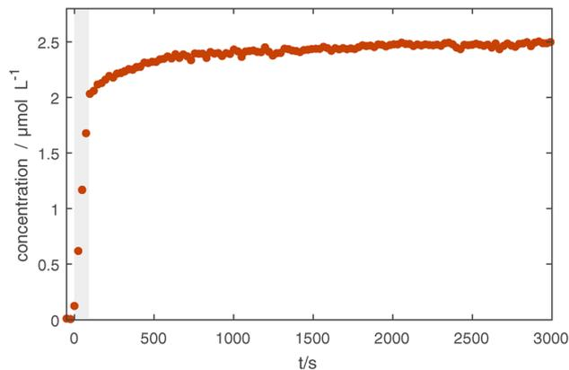
**Fig. 5** Prolonged argon plasma treatment of SiO<sub>2</sub>-coated Ag NPs. The particles have been generated in the GAS and coated using silane injection for 90 s (marked in grey) followed by an hour-long confinement. Gas pressure: 11 Pa, CCP power: 100 W, and argon flow: 30 sccm.
