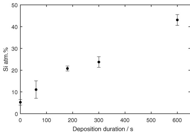
Fig. 8 Atomic concentration of Si measured with EDX during TEM measurements for extracted Ag@SiO<sub>2</sub> NPs with different coating times. Ten different areas of the TEM grid were used for statistical analysis. Only silver and silicon were taken into account to minimize the influence of oxidation after extraction and the background carbon support on the TEM grid.
