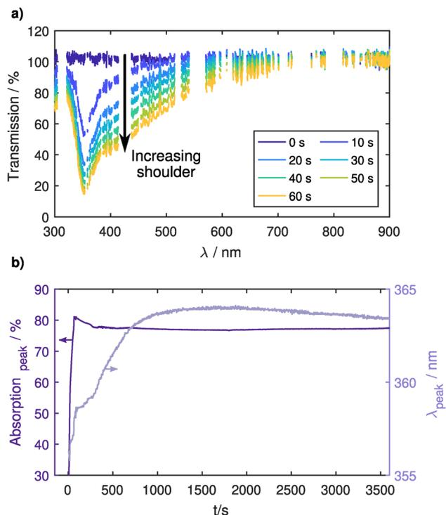
Fig. 2 (a) *In situ* UV-vis transmission spectra for 7 different times during the NP injection. 0 s corresponds to the plasma ignition in the GAS. At 60 s the injection of Ag NPs is stopped. Plasma emission lines were removed from the spectra. (b) Long-term measurement of injected Ag NPs, which are trapped for 1 h in the CCP plasma. The peak position  $\lambda_{\text{peak}}$  corresponds to the wavelength of the minimum in the transmission spectrum.
