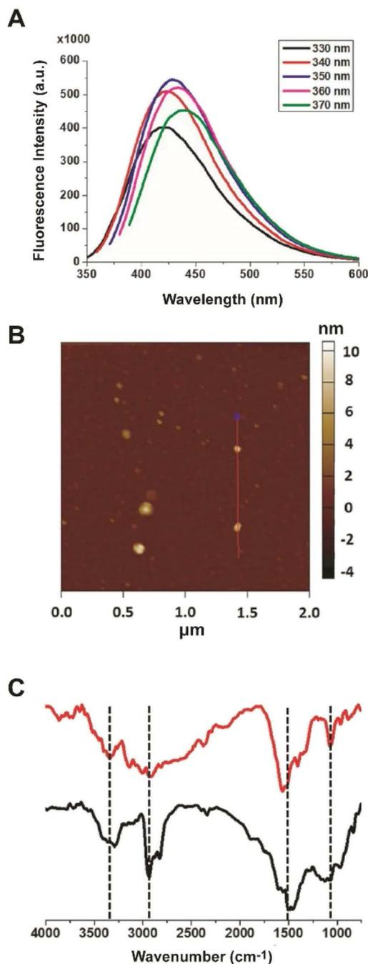
**Fig. 1** C-dot characterization. (A) PL emission spectra of the Lys C-dots upon excitation at different wavelengths (330–370 nm). (B) Representative AFM image showing Lys C-dots. The FTIR spectra (C) of the Lys C-dots. The peaks at  $\sim 3340$   $\text{cm}^{-1}$ ,  $2935$   $\text{cm}^{-1}$ , and  $1560$   $\text{cm}^{-1}$  are ascribed to N–H stretching, and the peak at  $\sim 1068$   $\text{cm}^{-1}$  is ascribed to C–N stretching.
