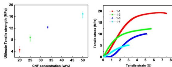
Fig. 10 Mechanical properties of zeolite-CNF composite films.
