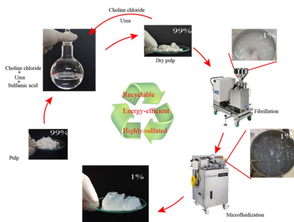
Fig. 1 Preparation process of sulfated CNFs.
