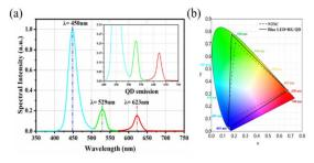
Fig. 5 (a) Emission spectrum of blue OLED backlight with a 50  $\mu$ m dual-color QDCCL. The inset is the same spectrum but with magnified red and green scales. (b) Color gamut diagram.
