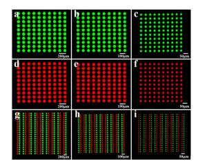
Fig. 3 (a–c) Green, (d–f) red and (g–i) dual-color QDCCLs with pixel sizes of  $90/50/20~\mu m$  prepared by SDA, respectively.
