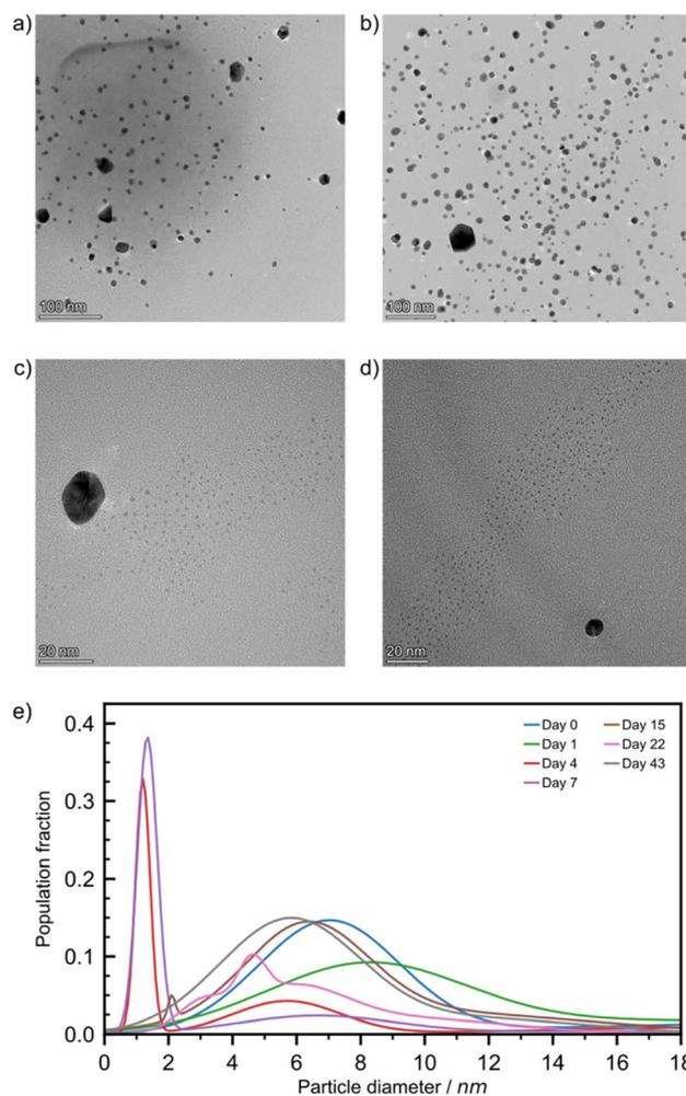
Fig. 4 Bright field TEM images from solution drop-cast preparation of the RT sample when aged for: (a) 0, (b) 1, (c) 4, and (d) 7 days at magnifications of  $\times 120k$ ,  $\times 94k$ ,  $\times 500k$ , and  $\times 390k$ , respectively. (e) The AuNP size population distributions for the RT sample after aging for 0 (blue), 1 (green), 4 (red), 7 (violet), 15 (brown), 22 (pink), and 43 (grey) days.
