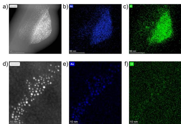
Fig. 5 Solid-state STEM-HAADF images and EDXS elemental maps for Au and Cl (left to right, respectively) for: (a–c) freshly milled powder at  $\times 186k$  magnification and (d–f) for the powder after seven days of aging at room temperature at  $\times 740k$  magnification.
