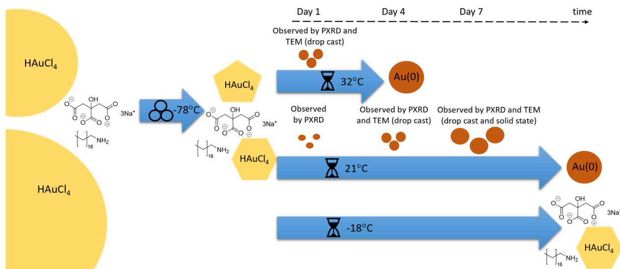
Fig. 7 Schematic representation of the synthetic sequence: precursors HAuCl<sub>4</sub>, NaT and ODA were milled at -78 °C, leading to HAuCl<sub>4</sub> comminution. Aging at -18 °C (LT) led to no reaction; aging at 21 °C (RT) led to gradual reduction and nanoparticle growth, as observed by different techniques; aging at 32 °C (ET) led to a similar outcome in an accelerated sequence.
