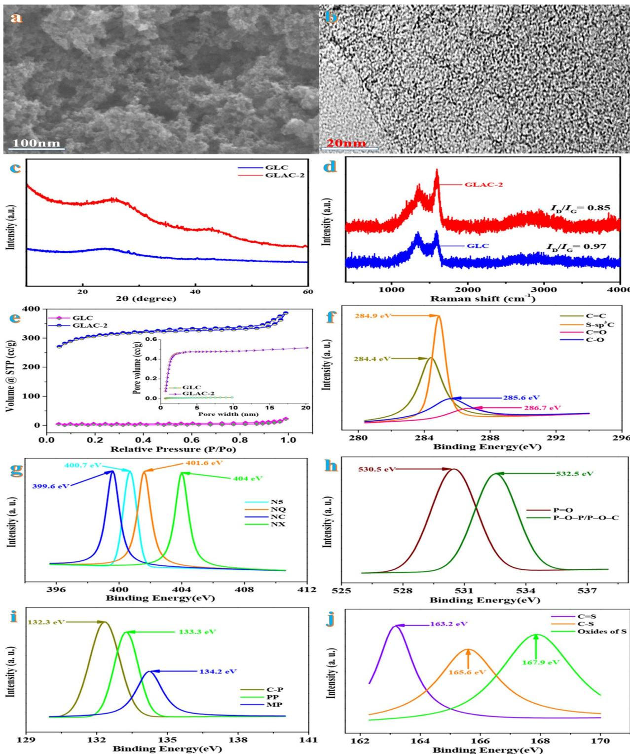
Fig. 1 (a) FESEM image of GLAC-2; (b) TEM image of GLAC-2; (c) XRD patterns of GLC and GLAC-2; (d) Raman spectrum of GLC and GLAC-2; (e)  $N_2$  adsorption/desorption isotherms and the pore size distribution of GLC and GLAC-2; (f) high-resolution C 1s of GLAC-2; (g) high-resolution N 1s of GLAC-2; (h) high-resolution O 2p of GLAC-2; (i) high-resolution P 2p of GLAC-2; (j) high-resolution S 2p of GLAC-2.
