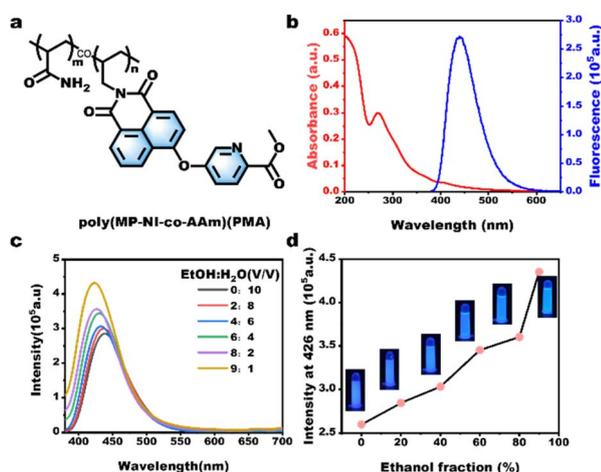
**Fig. 2** (a) Chemical structure of poly(MP-NI-co-AAm); (b) UV-vis and fluorescence spectra of aqueous PMA solution (0.01 M); (c) fluorescence spectra of PMA in mixed ethanol/ $\text{H}_2\text{O}$  solutions when excited at 365 nm; (d) peak fluorescence intensity of PMA as a function of the water content in mixed ethanol/ $\text{H}_2\text{O}$  solutions (inset photos showing fluorescence of PMA in mixed ethanol/ $\text{H}_2\text{O}$  solutions taken under 365 nm UV lamp).
