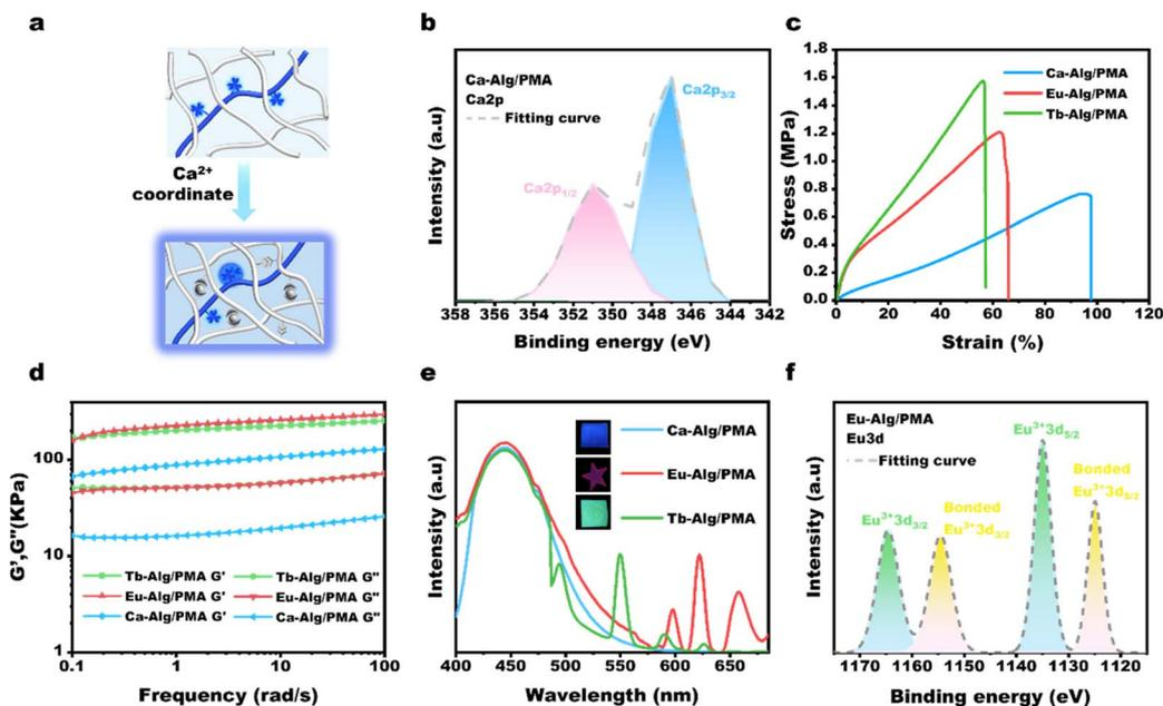
Fig. 3 (a) Scheme showing the preparation of dually cross-linked Ca-Alg/PMA hydrogels with  $\text{Ca}^{2+}$  coordination and hydrogen bonding crosslinks. (b) High-resolution XPS fitting spectra of Ca 2p; (c) tensile stress–strain curves; (d) rheology properties of Ca-Alg/PMA, Eu-Alg/PMA and Tb-Alg/PMA hydrogels at 1% strain; (e) normalized fluorescence spectra of the Eu-Alg/PMA, Tb-Alg/PMA and Ca-Alg/PMA hydrogels; and (f) high-resolution XPS fitting spectra of Eu 3d.
