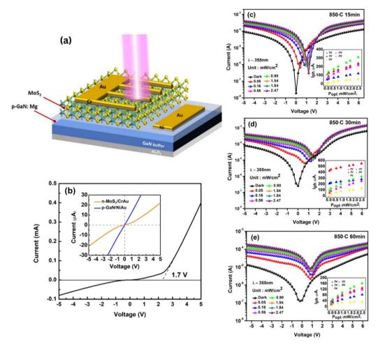
Fig. 5 (a) Schematic diagram of the  $n-MoS_2/p-GaN$  heterojunction photodetector. (b) Dark I-V curve of the  $n-MoS_2/p-GaN$  heterojunction photodetector and the metal-semiconductor contact properties (inset). (c-e) Photoresponse of the  $n-MoS_2/p-GaN$  heterojunction PD under varying light intensities. Inset shows the light intensity dependence of the photocurrent at different voltage biases.
