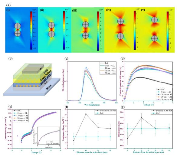
Fig. 4 (a) Simulation on the PNPs enclosed in a PEDOT:PSS envelope by COMSOL multiphysics. The distance (D) between the Au-NPs is varied and the simulation clearly shows the influence of surface coverage on the field coupling: (i) D=3 nm, (ii) D=5 nm, (iii) D=10 nm, (iv) D=20 nm and (D=10 nm, (D=10 nm,
