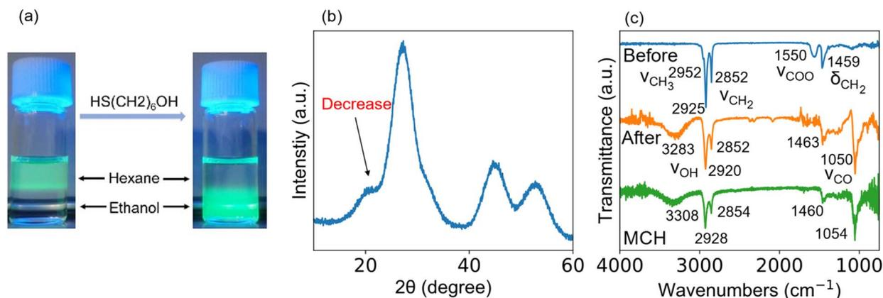
Fig. 2 (a) Photograph of the colloidal dispersion of InP/ZnS QDs before and after ligand exchange. (b) XRD pattern of the InP/ZnS QD capped with the MCH monolayer. The peak intensity at  $20^\circ$  decreased by the ligand exchange. (c) ATR-FTIR spectra of the InP/ZnS QD before (upper), after ligand exchange (middle), and MCH solution (bottom).
