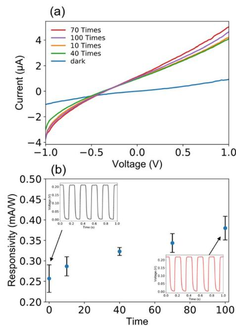
Fig. 5 Device lifetime of the MCH-QD-based photodiode measured at a voltage bias of 0 V at room temperature in ambient air using a  $470 \pm 5$  nm light with a power density of  $10 \text{ mW cm}^{-2}$ . Variation of (a) photocurrent and (b) responsivity for different number of measurements. Time response curves as insets were measured at the 1st time and 100th times. Error bars were obtained as the standard deviation by measuring 10 samples.
