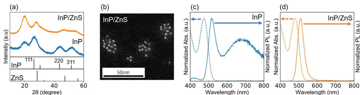
Fig. 1 (a) XRD patterns of the core InP and the coherent InP/ZnS core/shell QDs capped with PA monolayers. Standard peak positions of InP and ZnS were assigned using ICDD PDF 00-032-0452 and 01-071-5975. (b) HAADF-STEM image of the coherent InP/ZnS core/shell QD capped with PA monolayers. UV-vis and PL spectra of (c) the core InP and (d) the coherent InP/ZnS core/shell QDs capped with PA monolayers.
