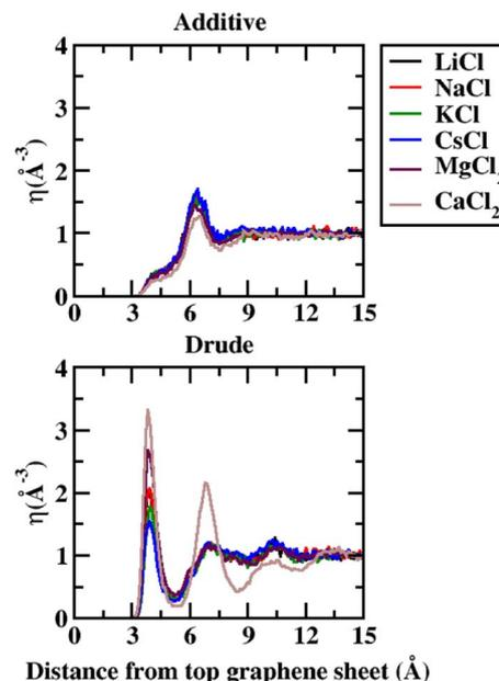
Fig. 4 Number density ( $\eta$ ) for  $\text{Cl}^-$  as a function of distance from the topmost graphene sheet, from 1 M additive and Drude polarizable FF salt simulations. All distances are presented in units of Å.
