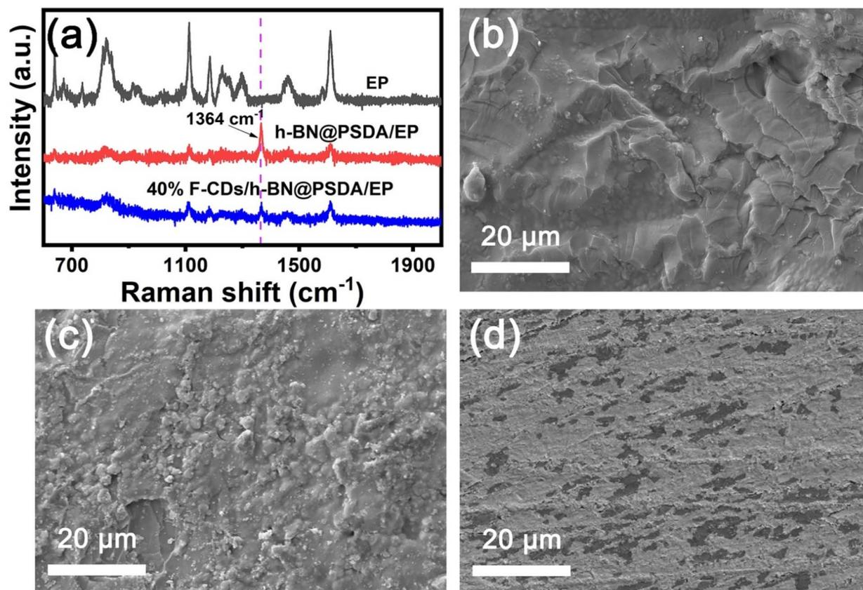
Fig. 8 (a) Raman spectra and SEM images of the worn surfaces of (b) neat EPs, (c) h-BN@PSDA/EPs, (d) 40 wt% F-CDs/h-BN@PSDA/EPs, respectively.
